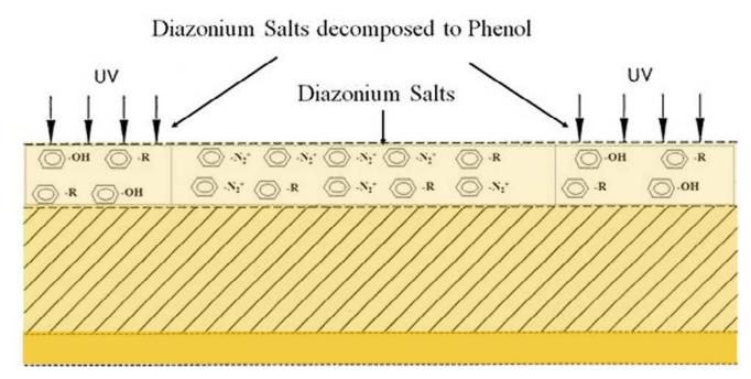
Figure 4: Diazo cross-section after exposure.
