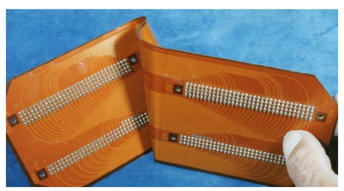
Figure 4: Four connectors: A three-layer FPC with central shield. Terminations are plated through and have soldered connectors.
