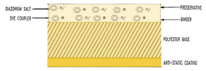
Figure 1: Structure of a typical diazo film.
