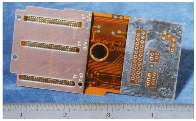
Figure 3: Stiffeners: FPC mimics PWBs when reinforced by an added structural layer; in this case (left end), epoxy-glass. The right end shows a ground plane or shield, which is part of the circuitry.
