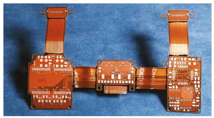
Figure 5: Rigid-flex circuitry provides the most space and weight efficient interconnection. This circuit has five rigid terminal areas with plated through-hole interconnections. Black material along the rigid edges is semi-hard and gives strain relief.
