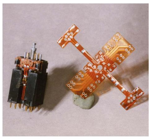
Figure 6: Relay circuit: FPC enables dense packaging. Relay on the left shows the FPC as folded/potted. The circuit is shown as manufactured on the right.
