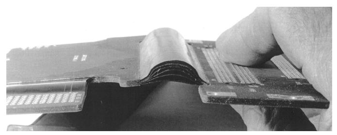
Figures 1 and 2: Bookbinder, shown flat (top) and bent (right). In rigid-flex circuits with bookbinder construction, which is very difficult to produce, FPC layers that will be on the outside of bent areas are designed slightly longer to provide ease in the formed position.
