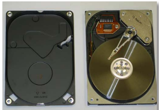
Figure 2: Little space is available and air flow is restricted—cooling from down and under the chip is the only solution.
