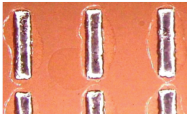
Figure 9: Printed and immediately reflowed.
