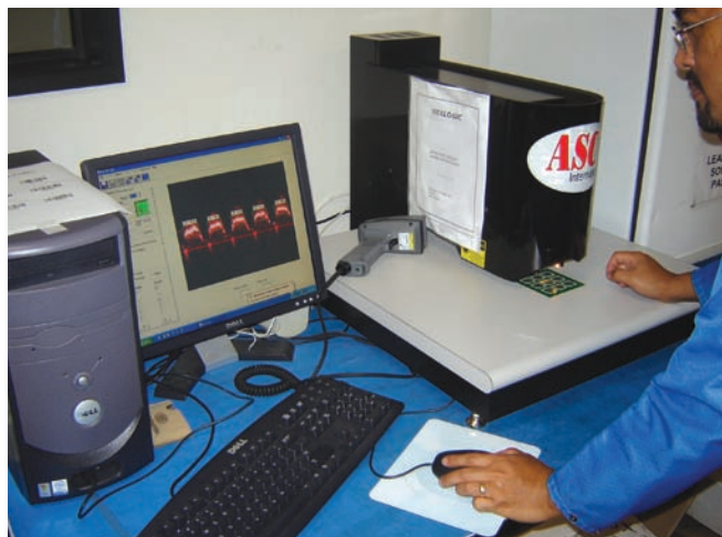
Figure 3: Paste height inspection verifies paste distribution on SM pad.
