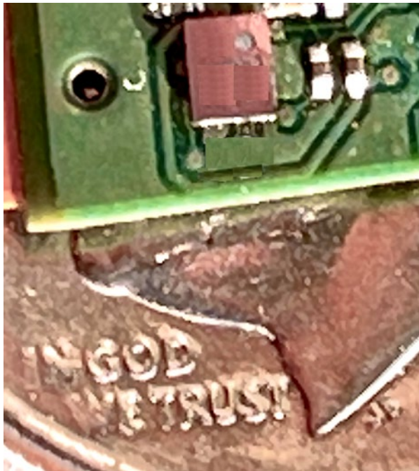
Figure 3: Extremely-dense PCB means minimal material usage, micro-scale packaging density; 0.24 mm pitch BGA shown presumed to exceed IPC producibility class C.
