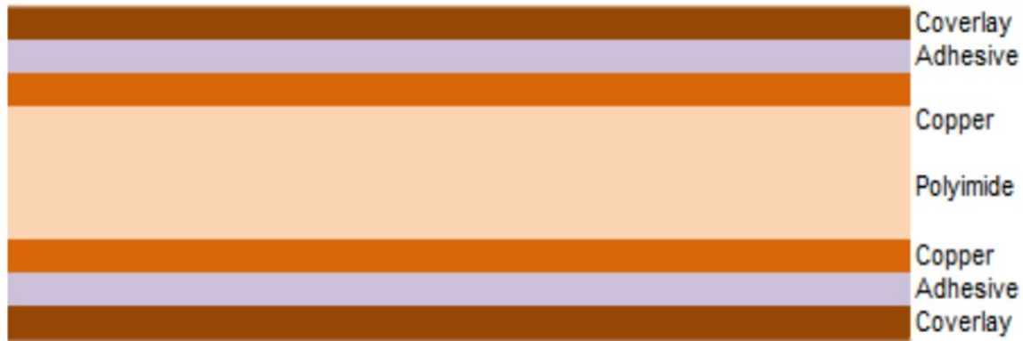
Figure 5: Illustration showing a two-layer construction with higher impedance requirements. The added thickness of the controlled impedance section makes circuits less flexible.
