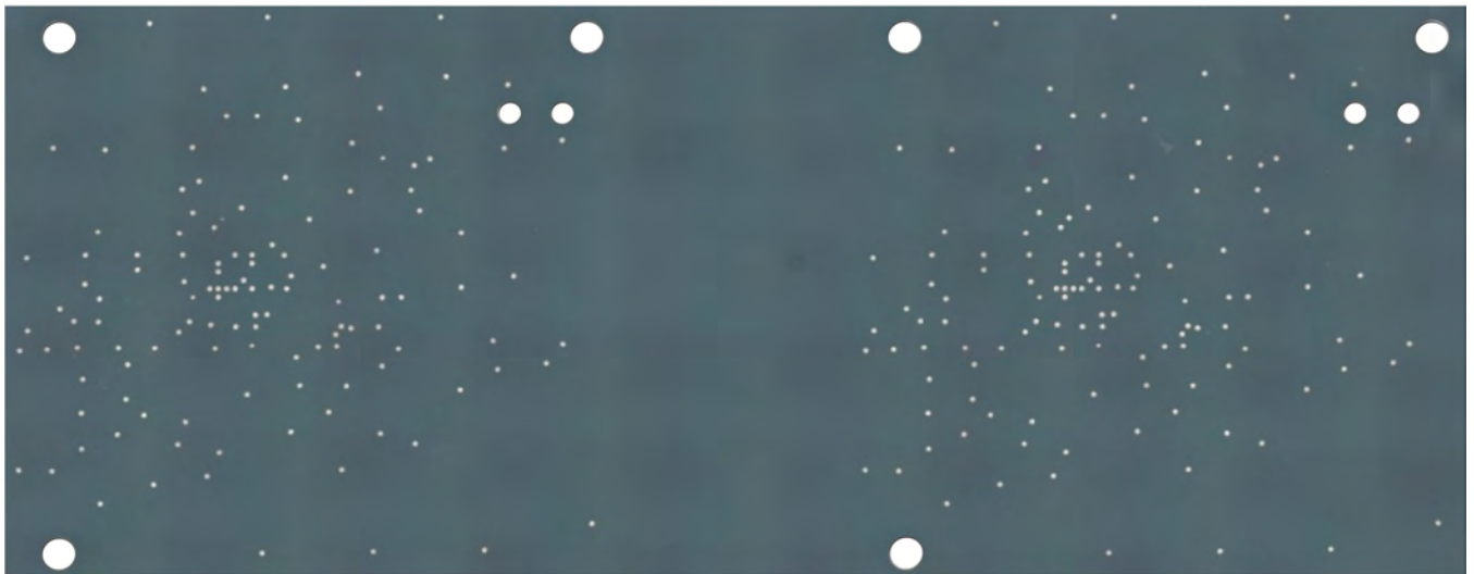
Figure 4: Screen-printed fiducials and reference pads.
