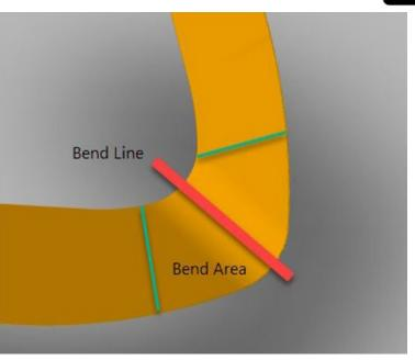
Figure 2: IPC-2581 Revision C also provides detailed information about the bend (type, direction, radius, and bend angle).
