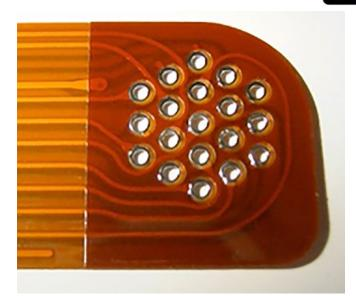
Figure 2: A 5-mil double-sided, thick cover coat used as a stiffener on a 1-mil very flexible circuit.
