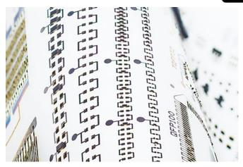
Mina is a simple pretreatment for aluminum that makes it as easy as soldering to copper.
