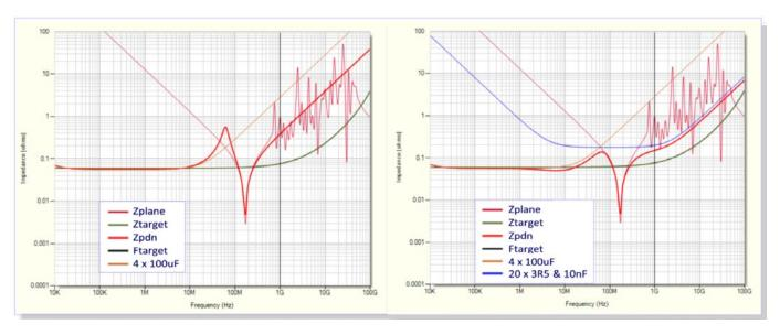
Figure 2: Zpdn with 4x100uF (left), Zpdn with added RC damping (right). (Source: iCD PDN Planner)
