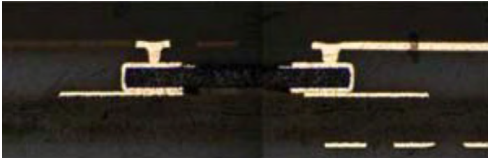
Figure 2: A 01005 microvia termination. (Source: IPC-7092)
