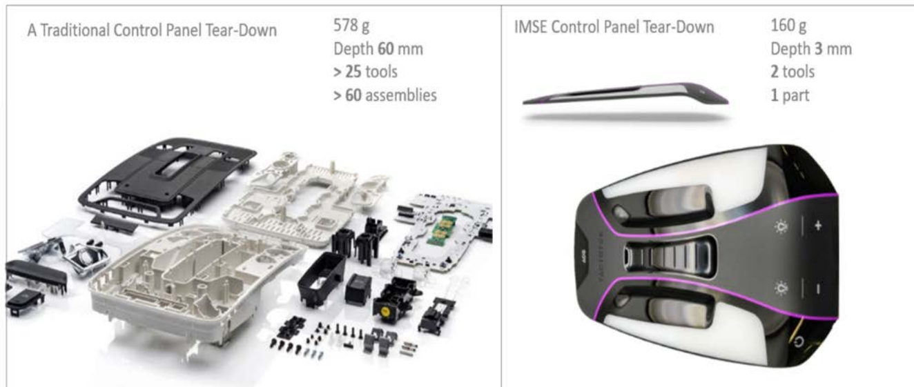
Figure 2: TactoTek has demonstrated structural electronics designs with 70% weight and 90% thickness reduction when compared with conventional multi-part assemblies.
