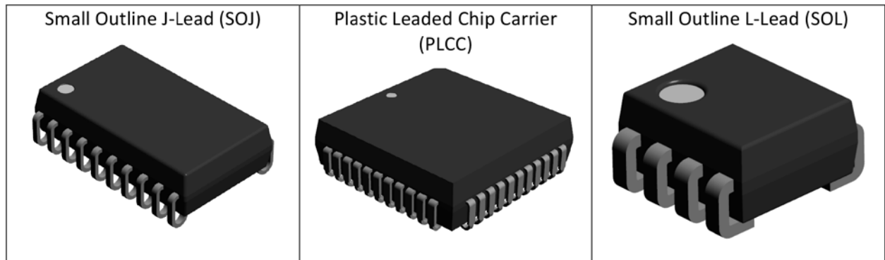
Figure 4: J-Lead & L-Lead Packages (SOJ, PLCC & SOL).
