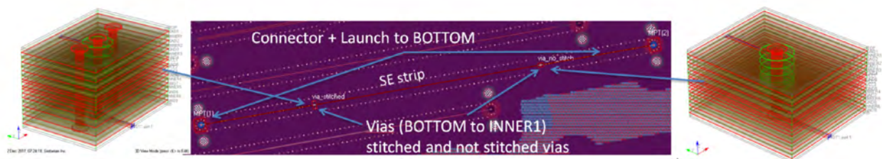
Figure 4: Two vias, one with two stitching vias and one without.
