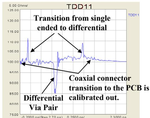
**Figure 2: TDR results comparing a Network Analyzer coaxial calibration versus a Single-Mode TRL calibration for the coupled differential via pair structure in Figure 1. The TRL calibration removes the connector discontinuity, but not the effect of transitioning from single-ended to differential transmission line routing.**
