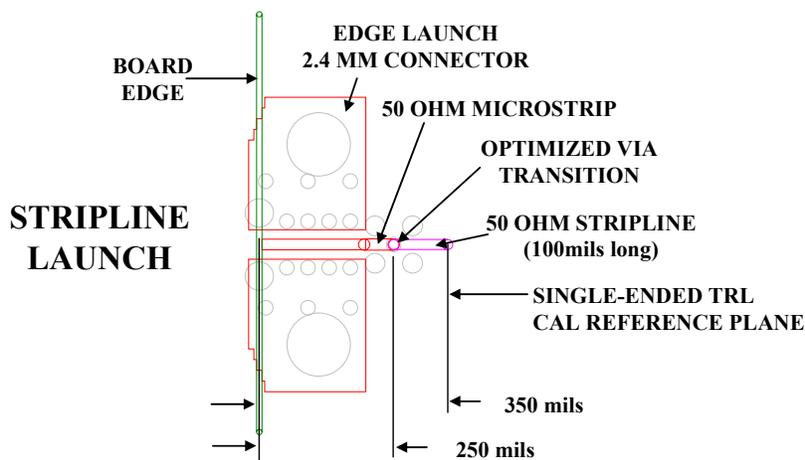
Figure 7: Single Ended Launch to Inner Layer Stripline
