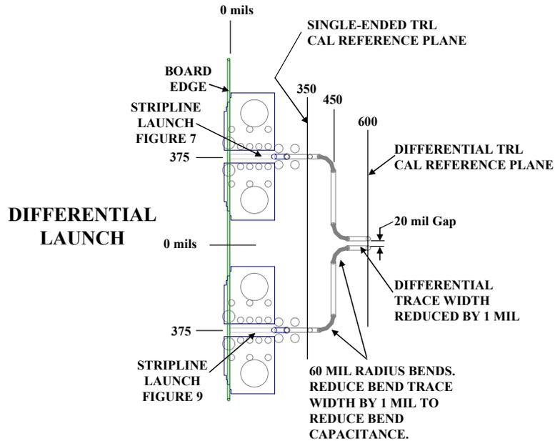
Figure 12: Differential Launch to Coupled Inner Layer Stripline – 4 Port
