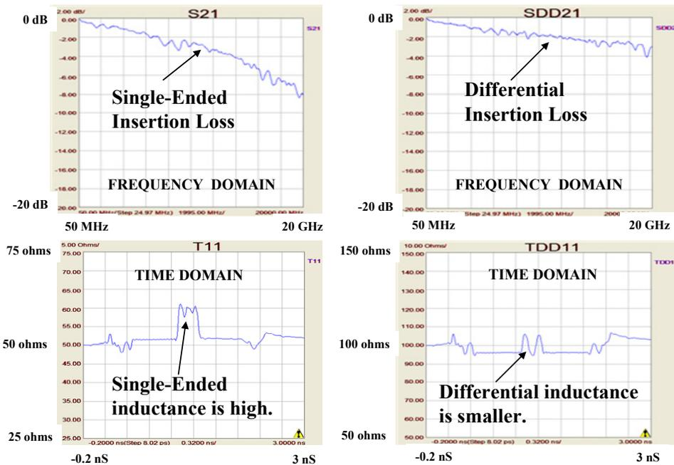
Figure 11: Single-ended vs mixed mode S-Parameters for the full-path structure of Figure 1.
