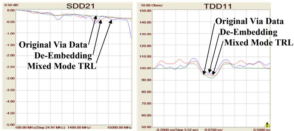
Figure 14: Simulated differential SDD21 to 15GHz and time domain TDD11 verification of the mixed-mode TRL and single-ended TRL with simulated feed-line de-embedding. Variations in the mixed-mode TRL show that the TRL structure through line is not long enough for the single ended to differential fields to settle resulting in a characteristic impedance that is different from that of a longer line.
