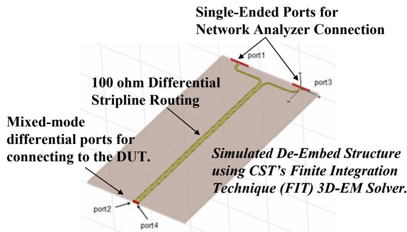
Figure 8: Example 3D-EM model of a feed line structure for connecting from the single-ended TRL reference plane to the DUT.
