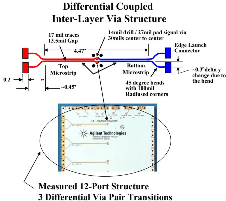
Figure 15 : Differential Via Experiments and TRL Calibration
