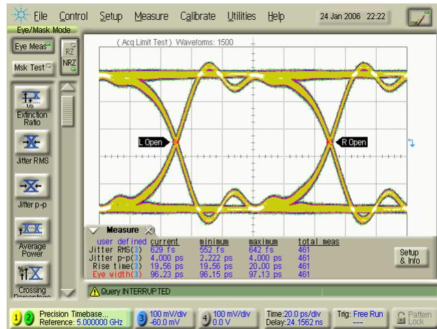
Figure 3 - Single Ended microstrip transmission line and measured data using a 10Gbps PRBS 31
