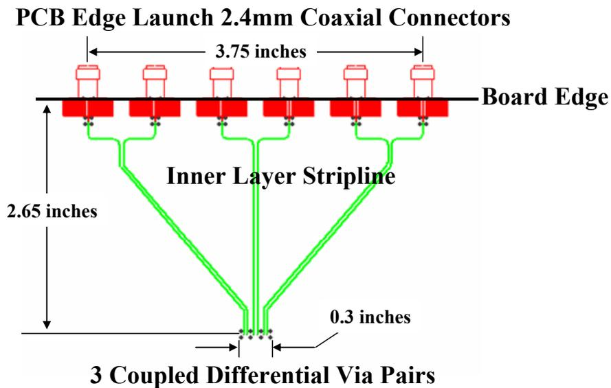
**Figure 6: 12-Port feed line routing to get from coaxial connectors to the via structure under test.**
