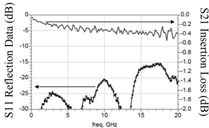
Figure 16: S-Parameter data for the Southwest 2.4mm PCB edge launch connector using *GigaTest Labs* probe measurements.
