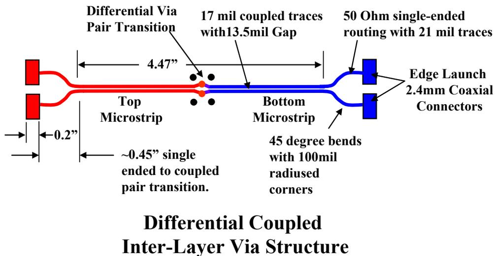
Figure 1: PCB layout showing the characterization problem.
