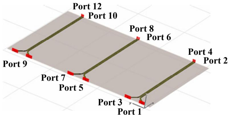
Figure 17: Simulated 12-Port de-embed microstrip structure.
