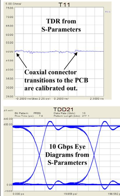
**Figure 4: Network Analyzer coaxial calibration vs single-ended TRL results for the microstrip trace in Figure 3.**
