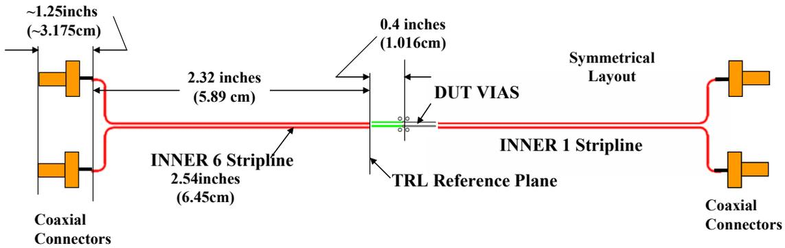
Figure 13: Simulated full-path structure and data for verification of the de-embedding and mixed-mode TRL algorithms.
