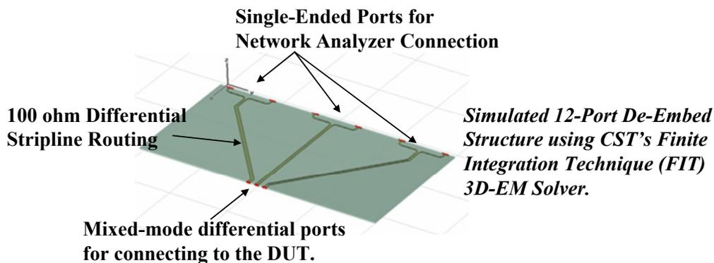
**Figure 9: 12-Port De-Embed structure showing the flexibility in routing to the DUT from the larger coaxial connectors.**
