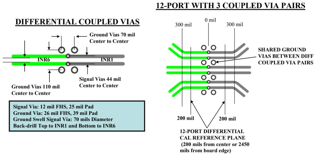
**Figure 5: 12-Port Differential Via Pairs for the DUT structure.**
