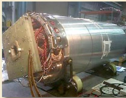
Dubbed HQ02a, the latest in LARP's series of high-field quadrupole magnets is wound with cables of the brittle, but high-performance superconductor niobium tin ( $Nb_3Sn$ ). Compared to the final-focus quadrupoles presently in place at the LHC, made with niobium titanium, HQ02a
