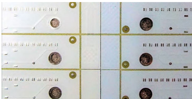
Figure 2: Different colors on two different types of solder mask.
