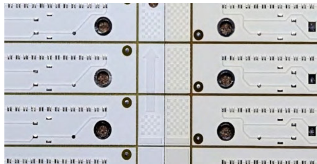
Figure 3: Solder mask "browning" with multiple reflow cycles.
