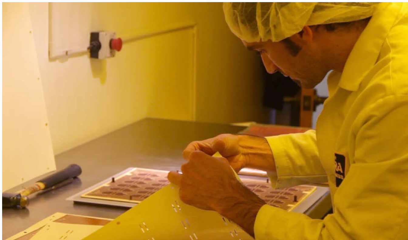
Figure 2: White acrylic adhesive layers are added to the lamination book. .....
