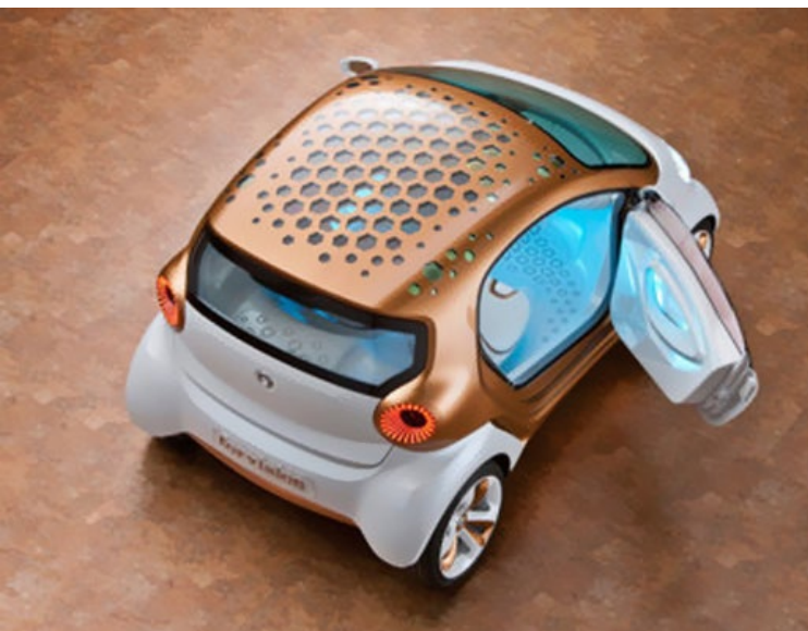
Figure 2: Car with printed organic light emitting diode OLED lighting on outside and inside of roof and printed photovoltaics over the outside generating electricity.
