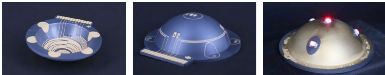
Figure 4: 3D MID examples (far right shows a functional 3D MID).
