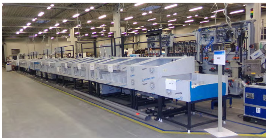
AWP Group's zero-liquid discharge, single-piece flow DES line under construction in Poland.
