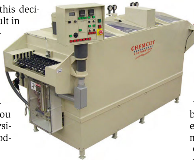
Figure 1: Example of a single-process line with etch (or other process), rinse and dry modules.
