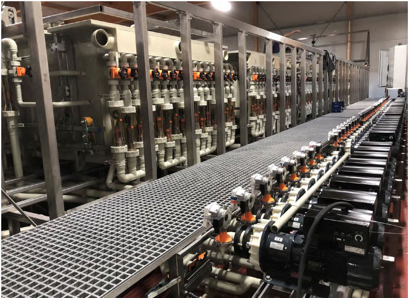
Ludy's zero liquid discharge specialized SAP and high aspect ratio plating line under construction in Germany.
