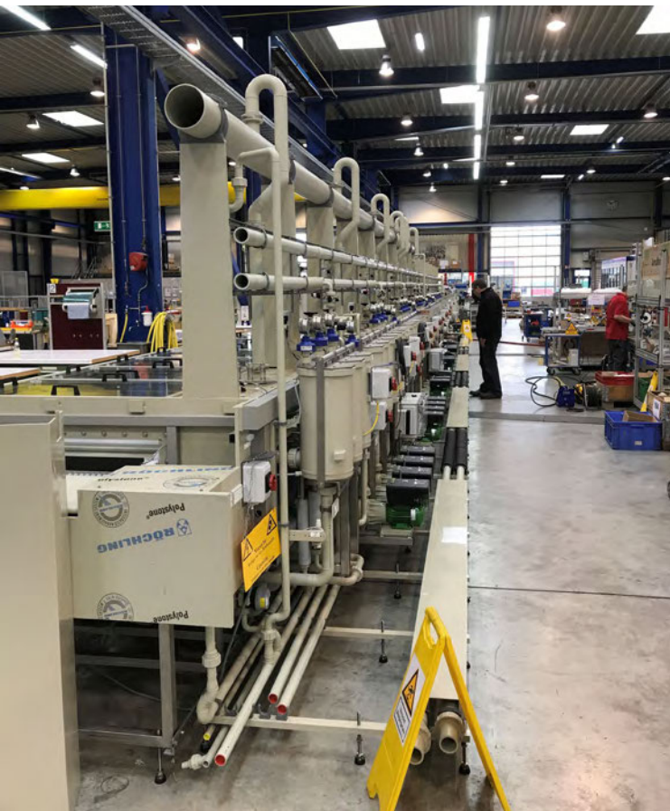
Atotech thin core flex electroless and flash plate line under construction in Germany.
