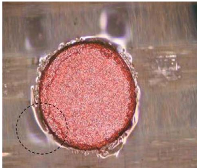
Figure 5: A laser drilled, paste filled via before lamination. Note the gaps in the glass fabric.
