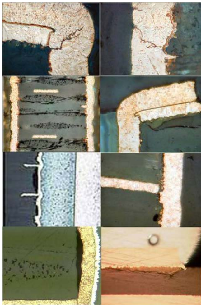
Figure 2: Cross-sectional micrographs of printed circuit defects caused by soldering are provided above. Clockwise from the upper left-hand corner: corner crack, barrel crack, pad lifting, post separation, pad cratering, hole wall pull away, resin recession and delamination.
