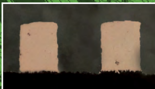
After CupraEtch DE Clean seed layer removal with no undercut
