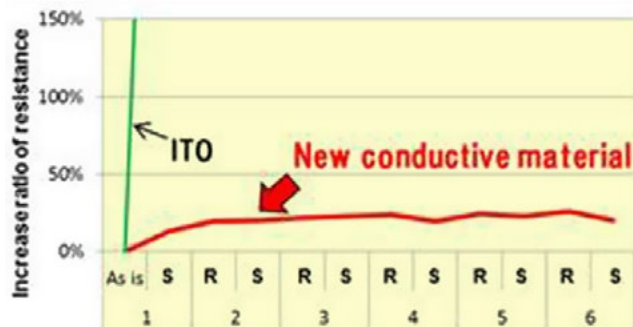
Figure 5: In comparison with ITO, the new conductive material which has been formulated offers superior performance.
