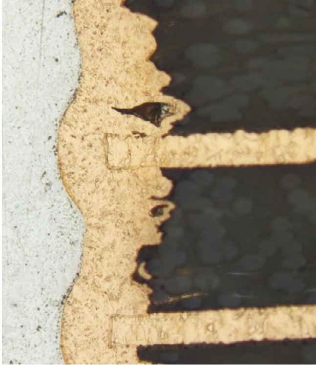
Figure 2: Excessive etchback leading to plating folds. Etchback exceeds 0.003 inches.
