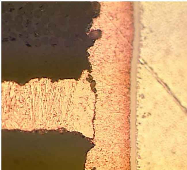
Figure 7: Note fine-line interconnect defect caused by drill smear that was not removed from interconnect.
