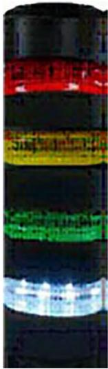
Figure 4: Example of an LED light tower with operation status (red, yellow, green) and interlock defeat status (white) LEDs.
