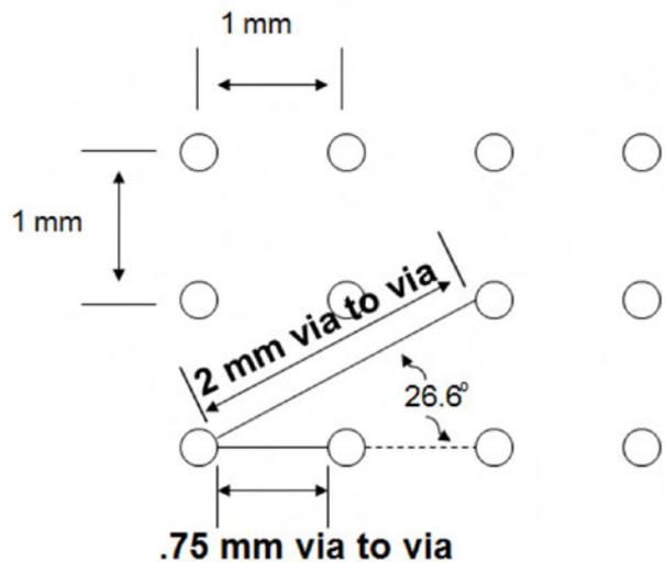
Figure 15: Via-to-via distance with rotated and non-rotated prepregs.
