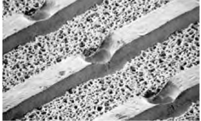
Figure 3: Landless via supplemented with the same diameter as the trace width, in this case, 0.004" (0.1 mm). These are referred to as 'invisible vias.' (Source: HP Sunnyvale PC)
