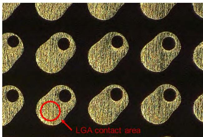
Figure 14: Via and LGA pad structure.
