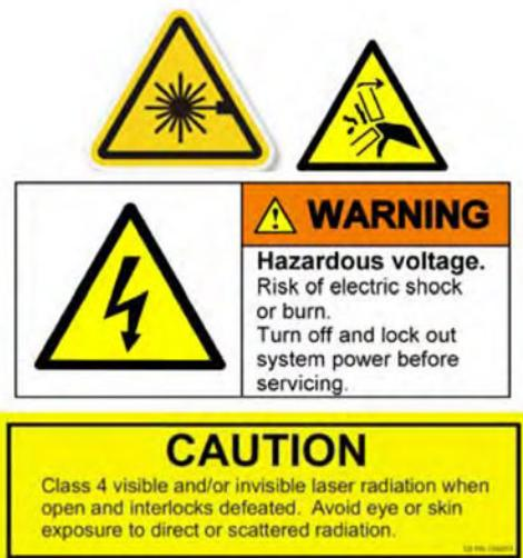
Figure 3: Examples of common laser system safety labels.
