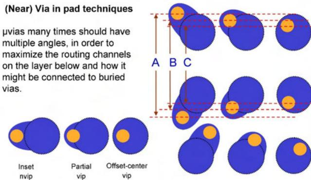
Figure 5: By ‘swinging’ the vias, depending on where the via is placed in respect to the SMT land, channels are created, A, B or C. These channels are the boulevards for 2X to 3X greater routing density<sup>[7]</sup>.
