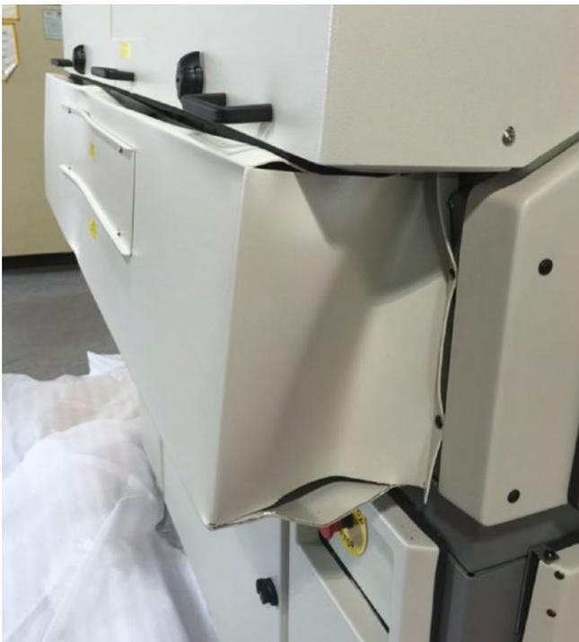
Figure 1: Poor handling during shipment can result in severe equipment damage.
