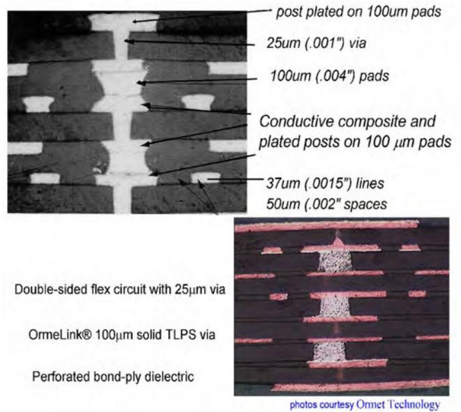
Figure 11: Examples of TLPS cross-sections of three layer pairs with lasered-vias filled with TLPS paste vias and buried vias for FR-4 innerlayers<sup>[8]</sup>.
