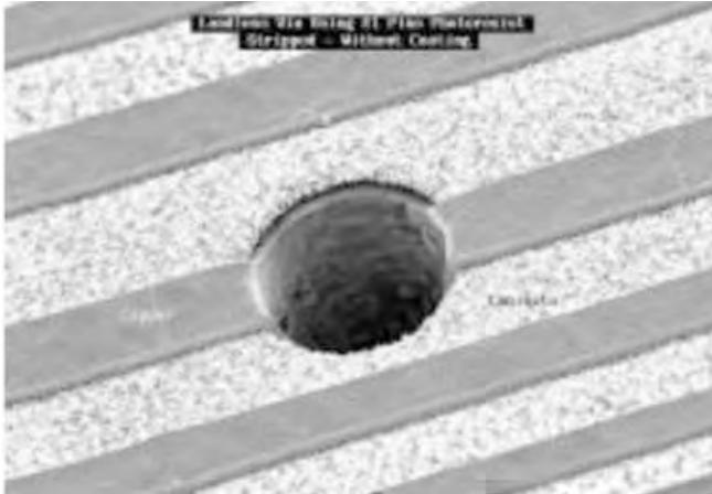
Figure 4: Landless via [0.010 in (0.25 mm) and .004 in (0.1 mm) traces] created with the liquid, electrophoretic, positive photoresist from PPG. (Source: Compunetics Inc.)
