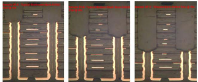
Figure 13: Microsection of three backdrill depths.
