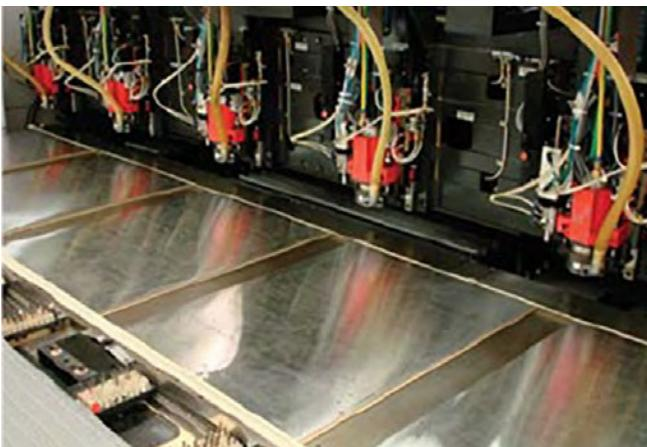
Figure 1: Five-head drilling machine.
