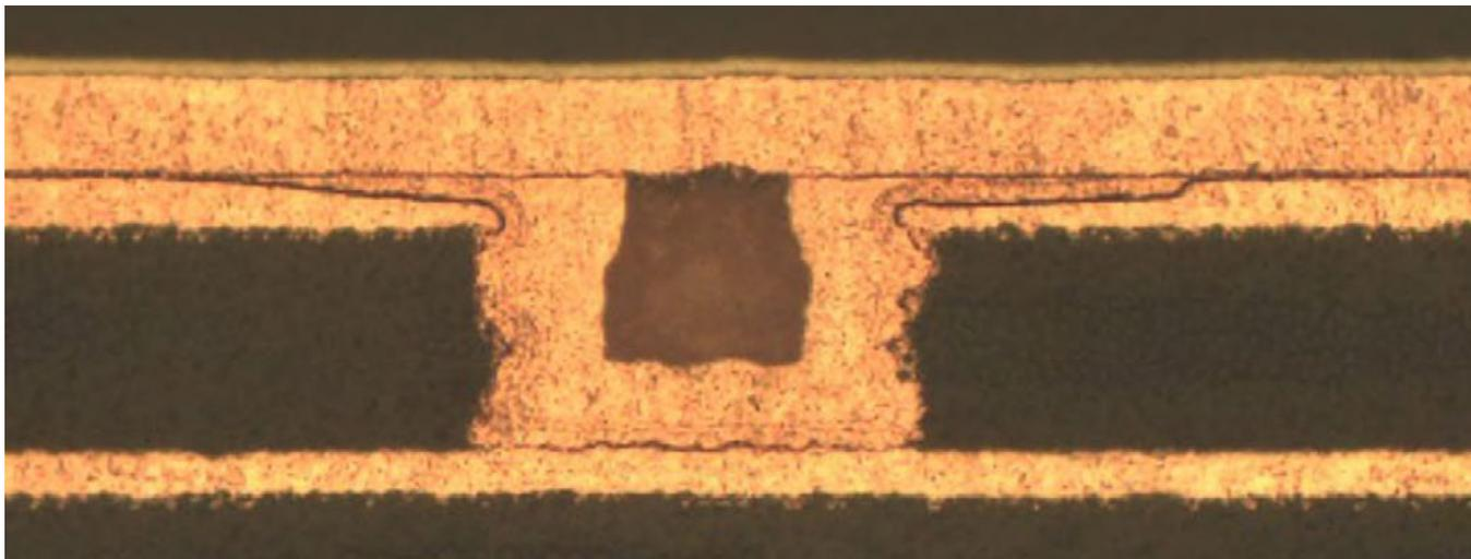
Figure 5: Filled microvia.
