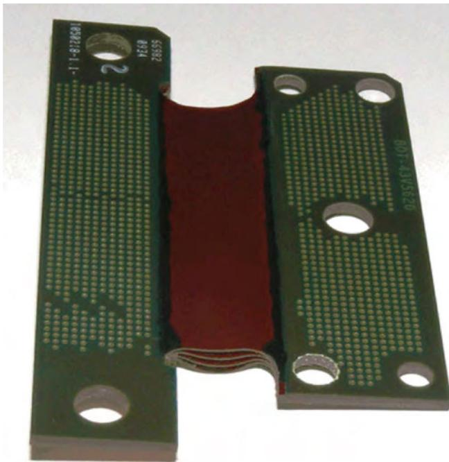
Figure 23: Rigid-flex with backside shown.
