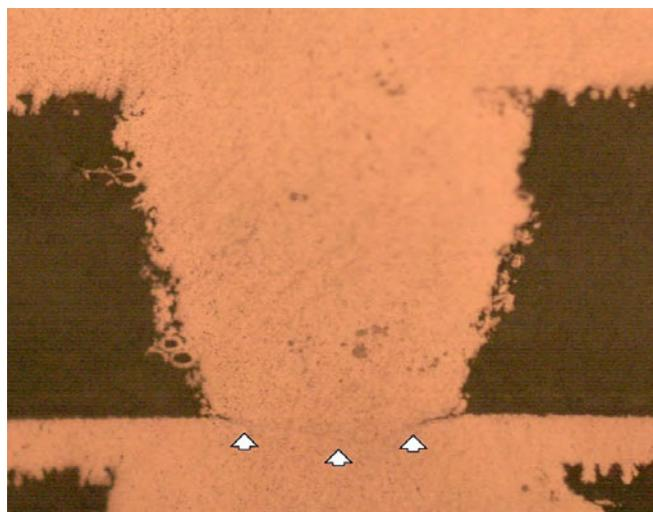
Figure 7: Separation in a microvia.
