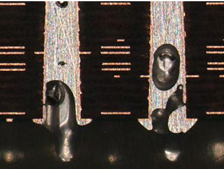
Figure 3: Large air pockets show where gas or moisture was expelled during the assembly process.
