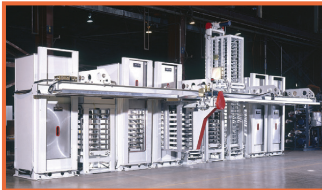
High Volume Press Systems with fully automated press loading and unloading
