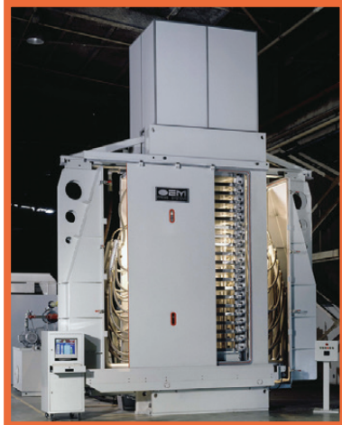
Copper Clad Laminate Vacuum Press Designed for full sheet production
