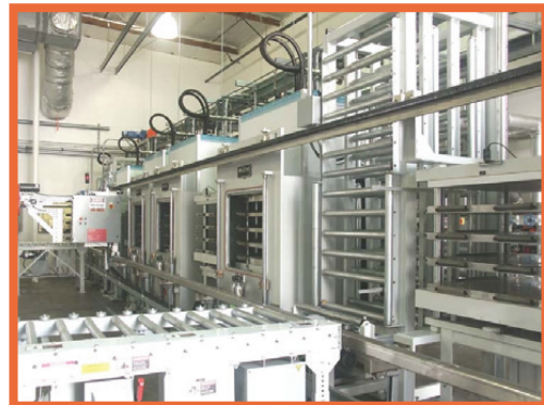
Quick-turn Vacuum Press Systems designed to accommodate high mix prototype production
