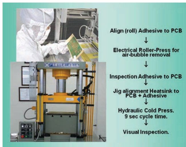
Figure 8: Adhesive attach process.
