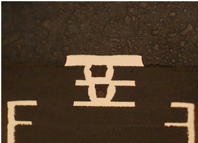
Figure 2: Plugged and capped microvia [2].
