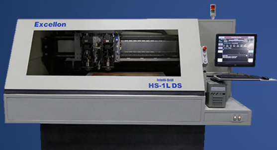
HS-1L DS Single-station, dual spindle high-speed system
