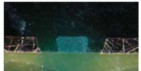
100µm solder dam, 40µm thickness on Cu
