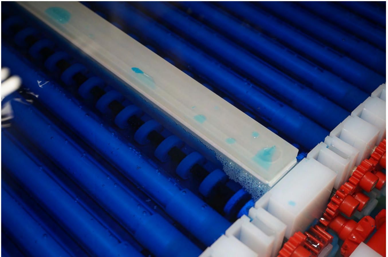
Figure 2: Very thin electroless plating processes from Atotech installed at GreenSource Fabrication.
