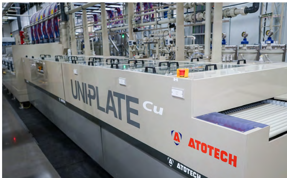
Figure 4: Atotech's world-renowned Uniplate IP2 advanced copper plater.
