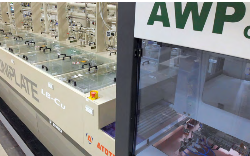
Figure 3: The Atotech electroless copper line (Uniplate LB) and copper plater (Uniplate IP2) on site at GreenSource Fabrication.
