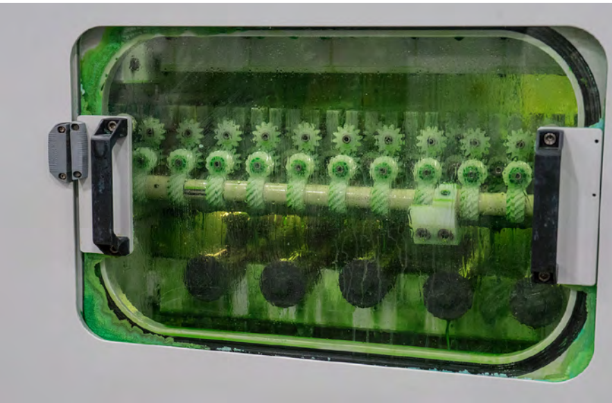
Figure 4: Wet-etch processes utilize bottom-side etching for greater efficiencies.
