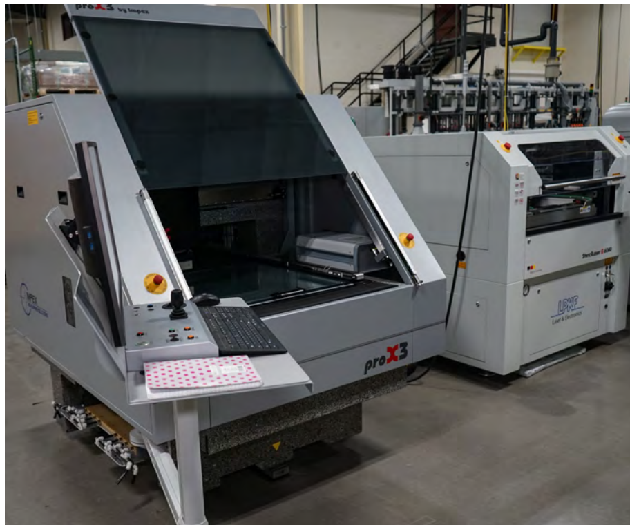
Figure 6: The Impex Measuring Solutions proX3 quality inspection and test tool at GreenSource Fabrication.
