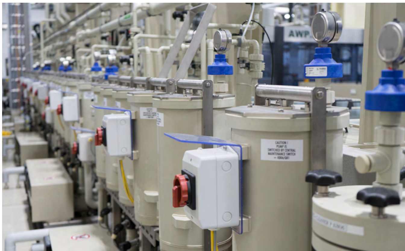
Figure 9: Back-side view of modules with fine particle filtration units.
