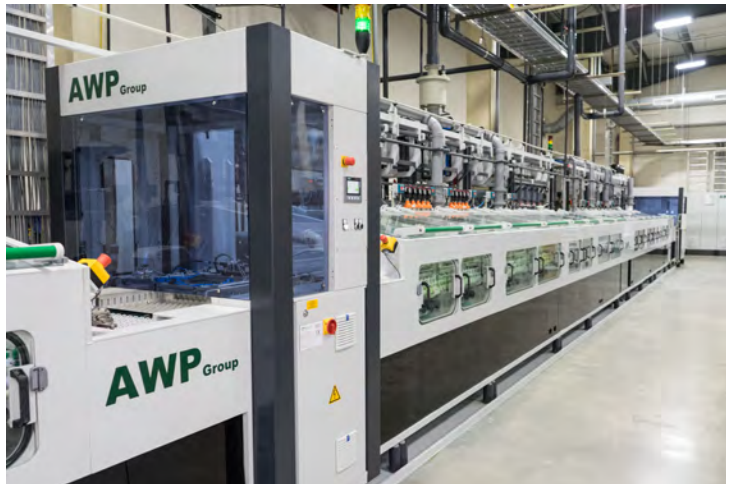
Figure 8: AWP’s innovative panel flipper enables back-to-back bottom etching for both sides of the panel.
