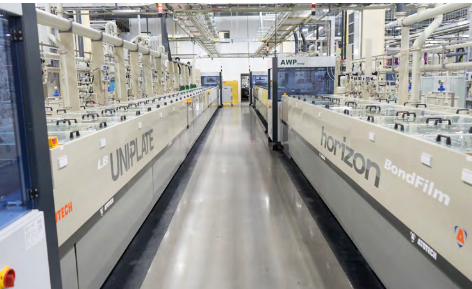
Figure 2: Atotech's horizontal production lines installed at GreenSource Fabrication (left: electroless copper line; right: oxide replacement line).
