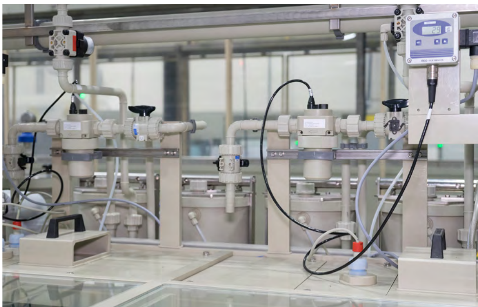
Figure 5: Supply pipes from above for recycled water. Control devices and sensors.
