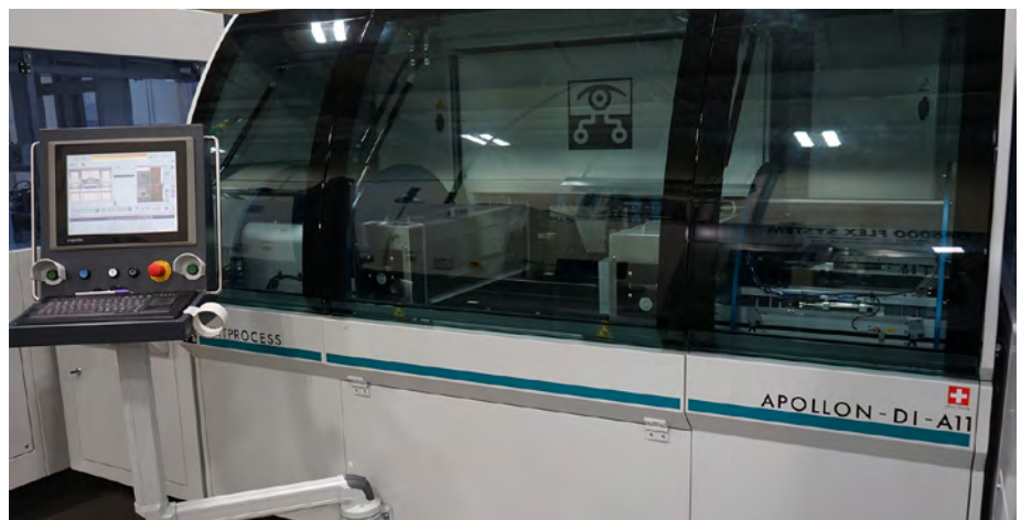
Figure 5: Apollon digital direct imaging system, auto-reverse inline.
