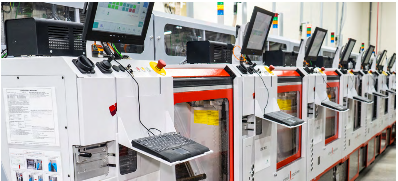
Figure 8: This bank of Schmolz Modul series drilling machines are outfitted with 3D back-drillings boxes.
