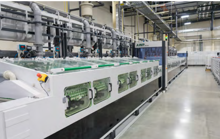
Figure 2: AWP's wet etch line installed at GreenSource Fabrication.
