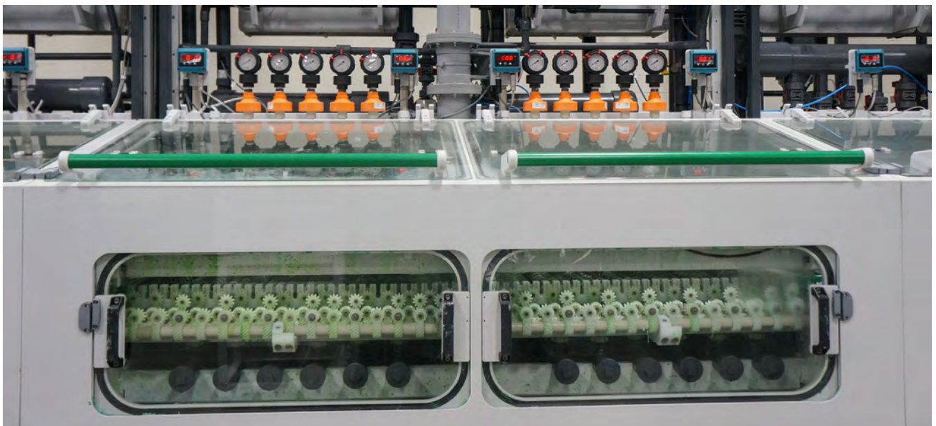
Figure 1: GreenSource Fabrication's automated wet etch uses AWP etching and material handling equipment.
