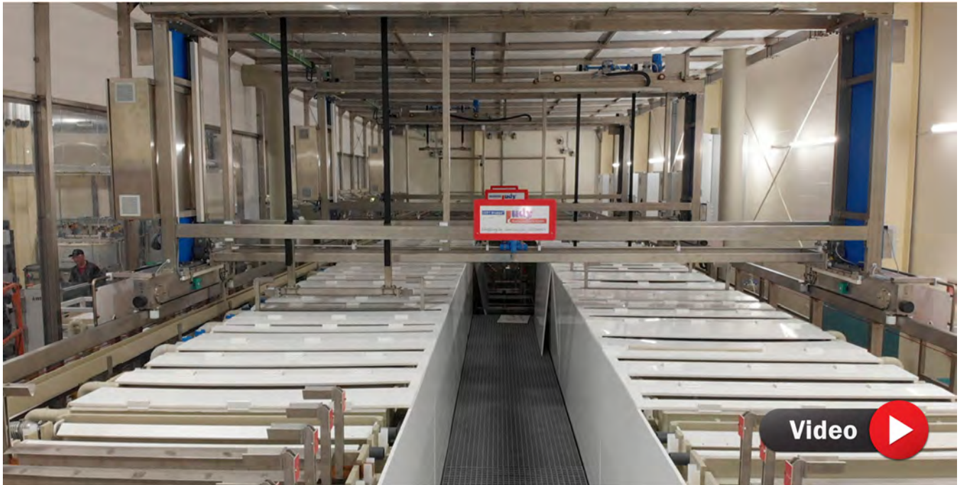
Figure 3: The Ludy vertical line at GreenSource shown here is nearing completion. Once operational, it is expected to be capable of microvia aspect ratios up to 40:1 and beyond. Click to watch flyover drone video.
