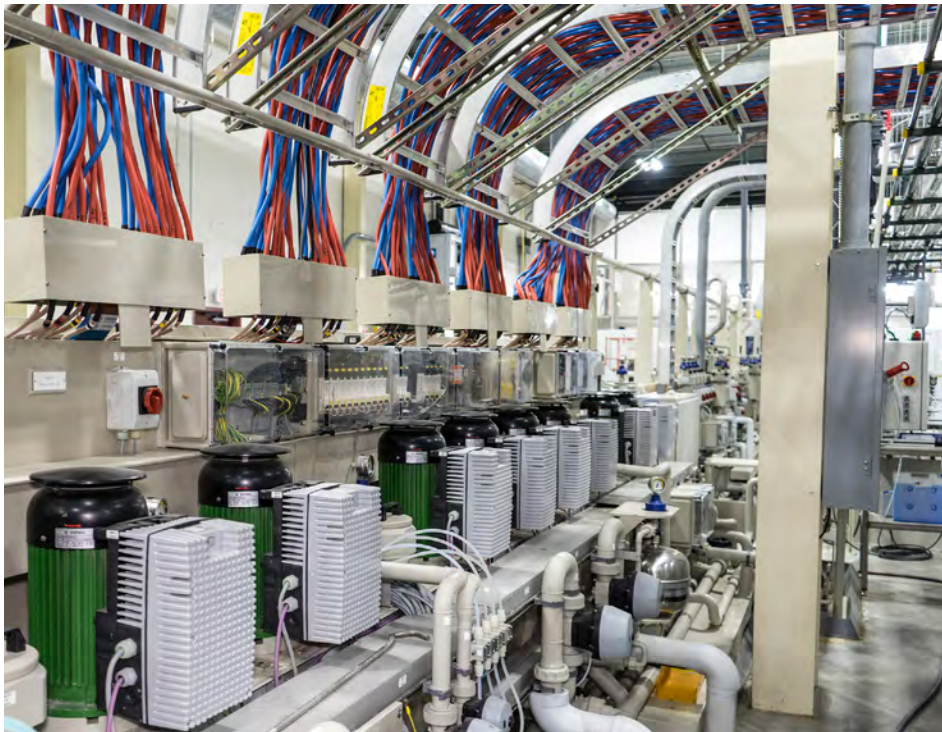
Figure 6: Back-side view of the Uniplate IP2 advanced copper plater showing frequency-controlled circulation pumps.
