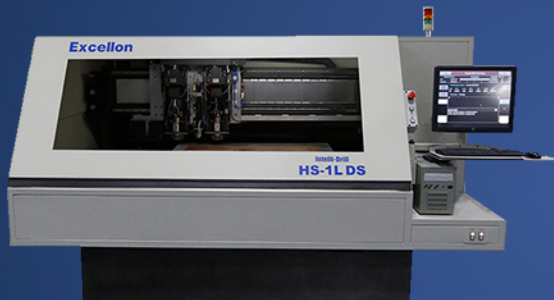
HS-1L DS Single-station, dual spindle high-speed system
