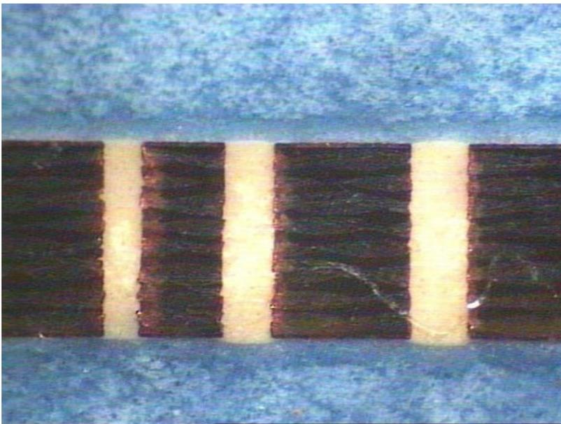
Figure 1: Example of a paste-filled through-hole.
