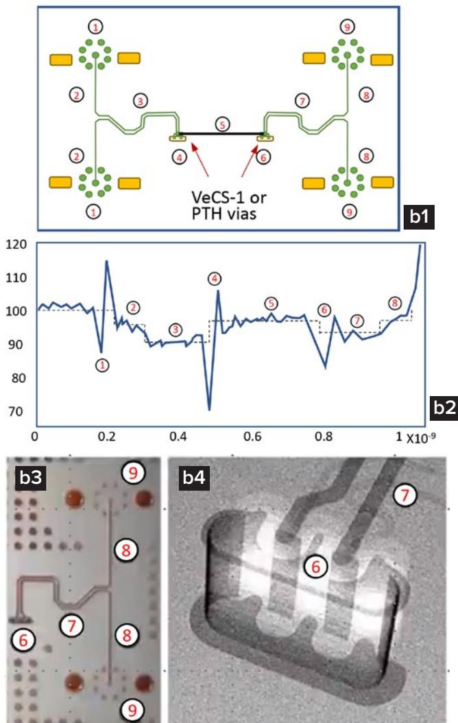
Figure 7b: Four figures of a high-speed signal propagation (impedance) through the back-drilled VeCS-1 connections;
