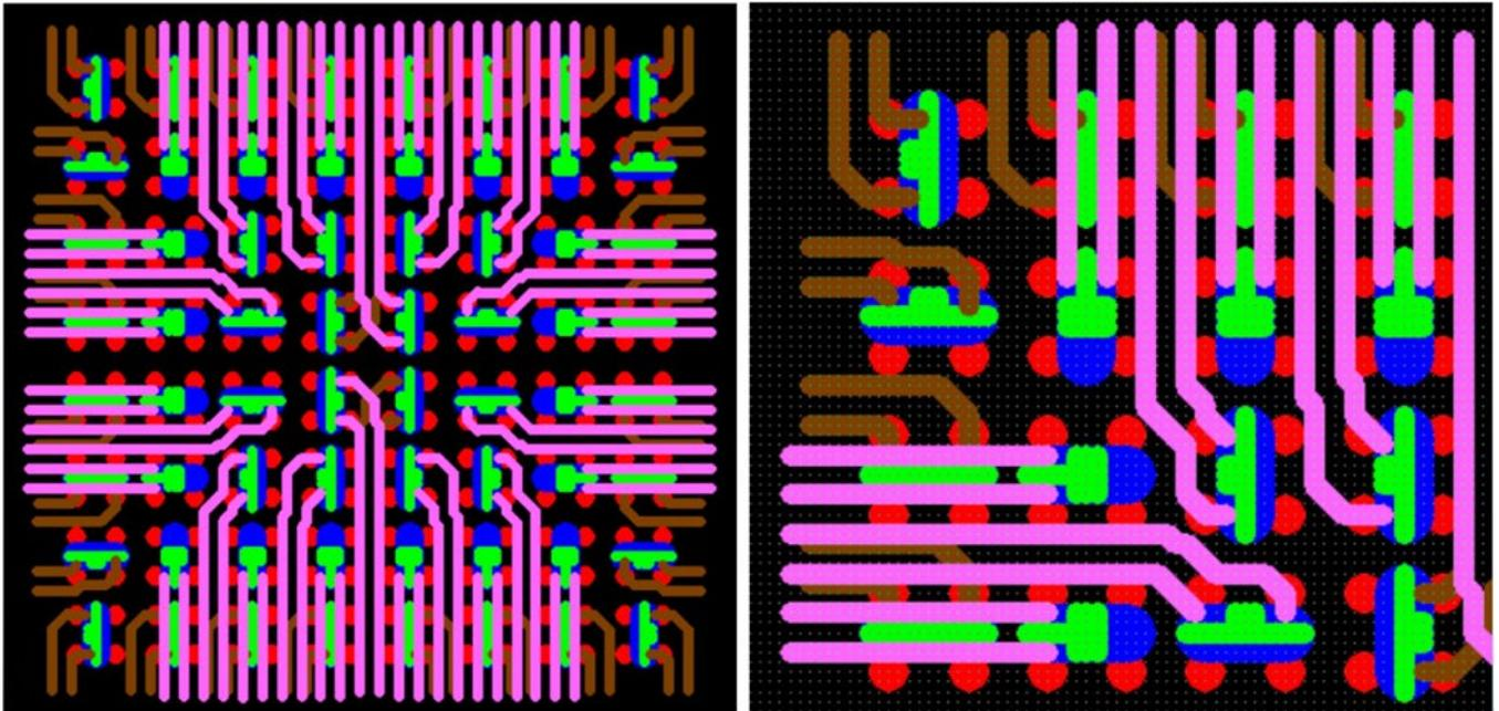
Figure 10: Routing of a very-fine pitch BGA using HDI, and VeCS-2 buried slots with close-up of quarter-pattern. (Source: NextGIn Technologies)
