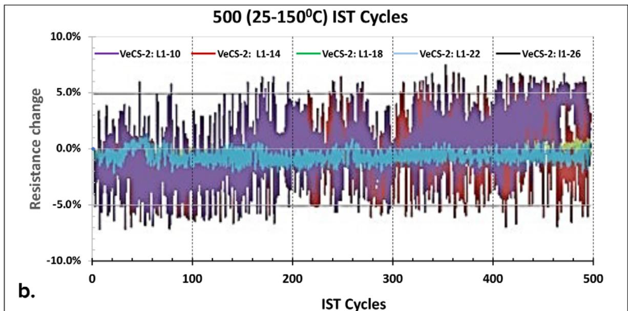
Figure 8: a) CAF test of three VeCS structures for 1090 hours at 85% RH, 85°C at 100 volts; b) resistance change of five VeCS-2 slot structures for 500 cycles of 25 to 150°C. (Source: WUS Printed Circuit Co.)
