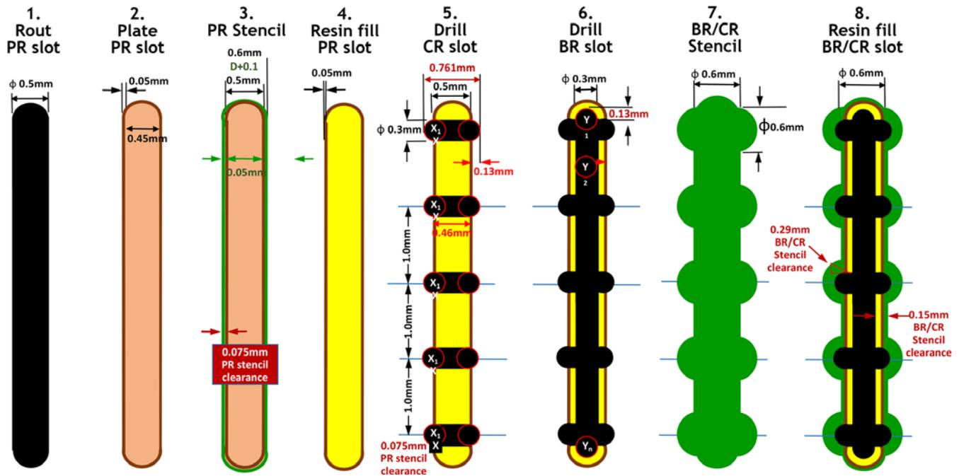
Figure 5: The VeCS fabrication eight-step process<sup>8</sup>. (Source: NextGIn)
