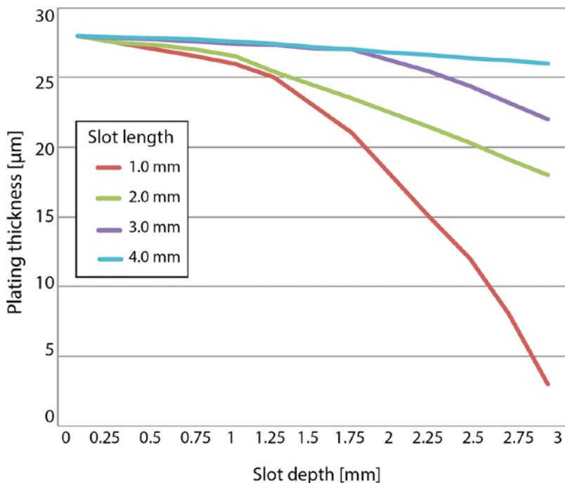
Figure 4: Plating thickness as a function of slot depth and length<sup>3</sup>. (Source: NextGIn)
