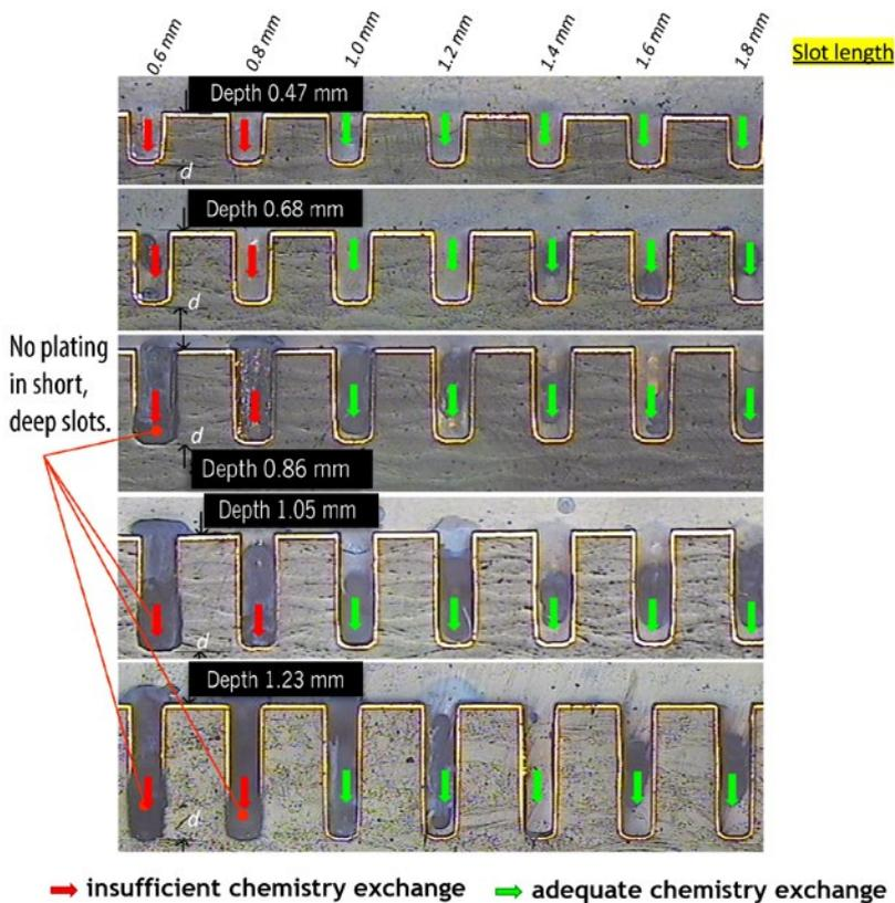
Figure 3: Creating and plating the blind channel (slot) is the key feature of VeCS-2 but is within the capability of any high-performance PCB fabricator<sup>3</sup>. (Source: NextGIn)
