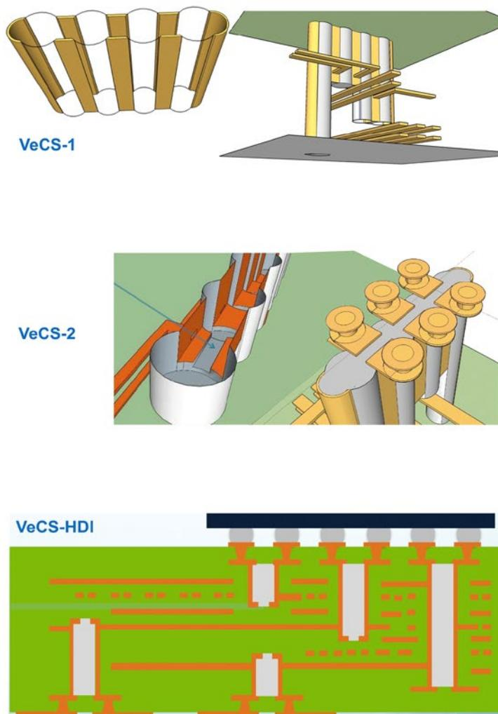
With channels (slots) formed from both sides, the 3D vertical traces provide greatly increased density without sequential laminations. Replacing larger through-hole vias with slots provides better power integrity for new power-hungry chips while lowering inductance and capacitance for improved signal integrity.
