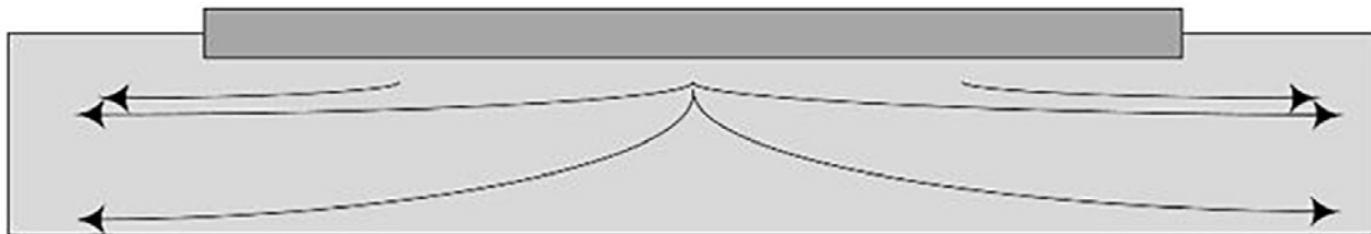
Figure 4: The cooling path for a trace is longer from the center of the trace than it is from the edge of the trace.
