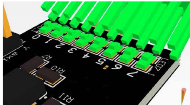
Figure 5: Simulated bending of a flex circuit reveals a clearance violation between a flex-mounted pin-header and SMDs on the main rigid board. The violating components are highlighted green.
