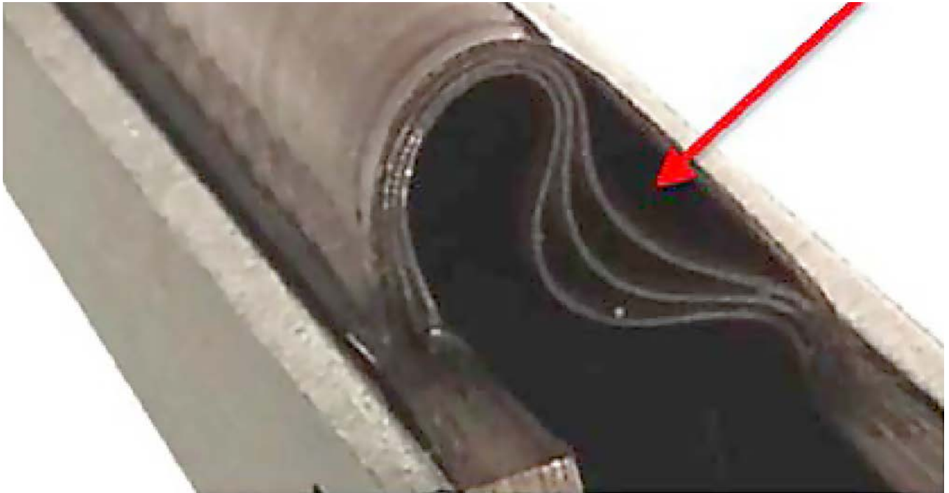
Figure 3: In this commercially produced design, the designers obviously did not apply bookbinder construction, resulting in additional stress on the separated layers (red arrow).
