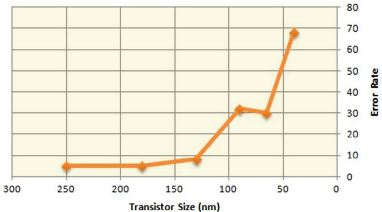
Figure 1: Transistor size vs. microprocessor error rate (source: Oracle).
