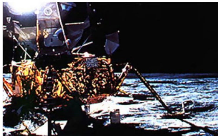
Figure 2: Gold foil acts as a radiation shield on the Apollo lunar module (courtesy of World Gold Council).
