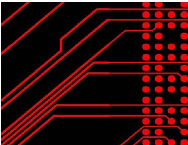
Figure 1: This could easily have been routed with 100 \mu m tracks and gaps outside the BGA pins.
