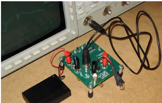
Figure 4: Setup with an RG178 50-ohm coaxial cable.
