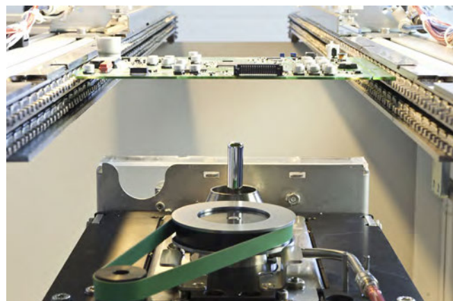
Figure 3: A wettable nozzle on an inline selective soldering machine.
