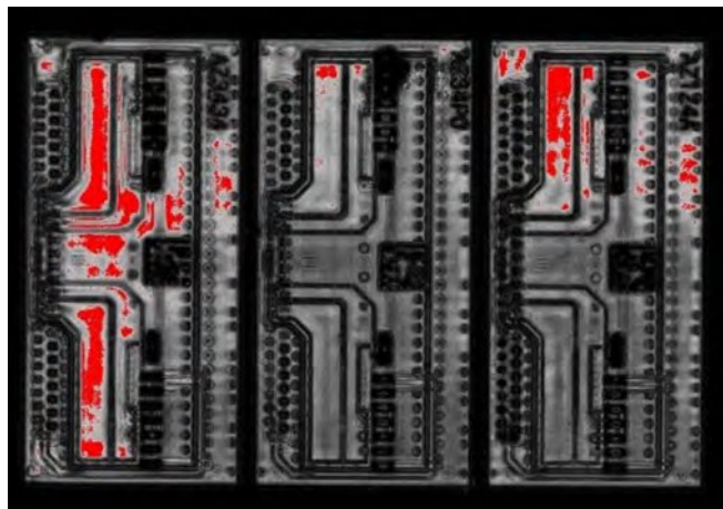
Figure 7(e): C-scan image from Gate #5, UF2, organics interfaces at 100MHz probe frequency. Both left and right units show significant delamination or less material regions.
