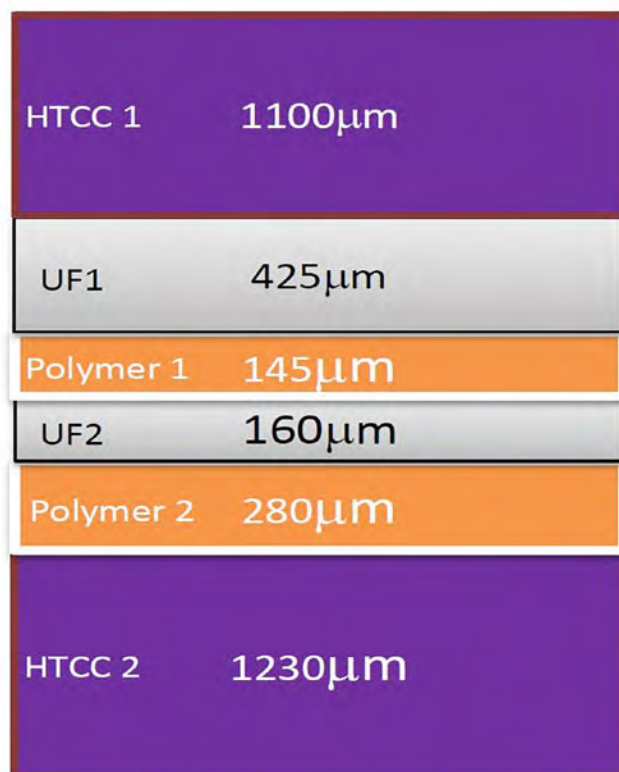
Figure 1: Illustration of material structure of the sample and their thickness in micrometer. Outer layers are high-temperature, co-fired ceramics.
