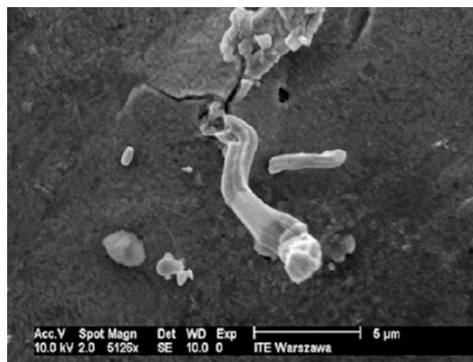
Figure1: SEM images of the samples soldered directly on Cu layer after 3000 h exposure at 87% RH and 60°C—the edge of the solder area. (A) Sn100, (B) Sn99.3Cu0.7Ni.
