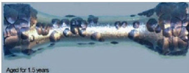
Figure 8: Plumbridge's photo of tin pest forming on a tensile specimen stored at 18°C for 1.5 years.
