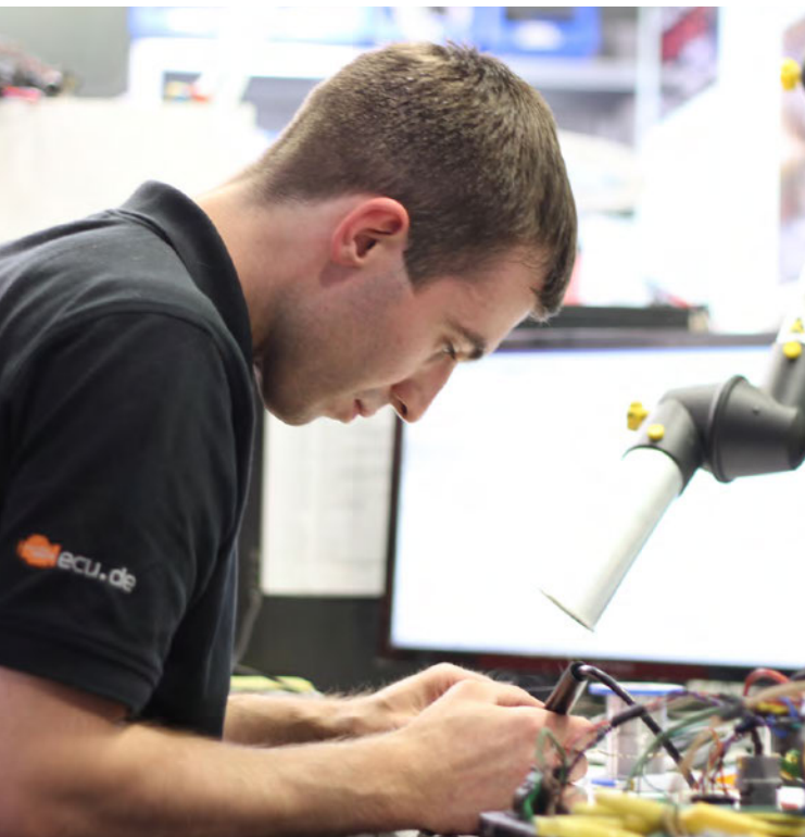
Figure 2: Fume extraction setup for hand soldering processes.
