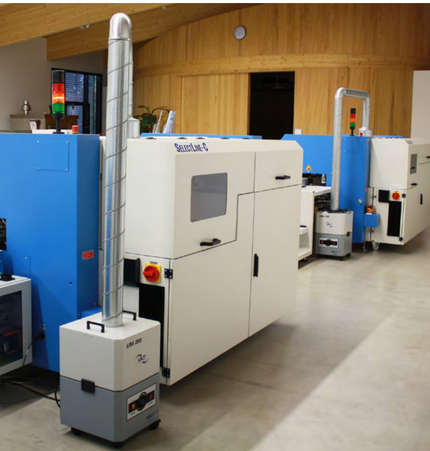
Figure 1: ULT offers a versatile extraction and filtration system for the efficient removal of soldering fume.
