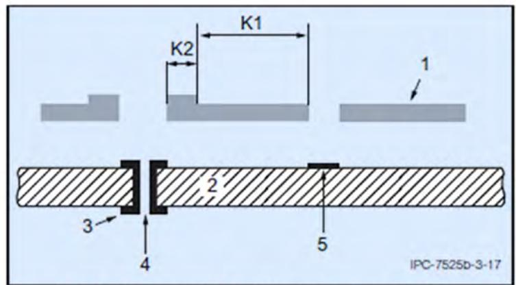
Figure 3-17 Overprint With Step (Squeegee Side)
