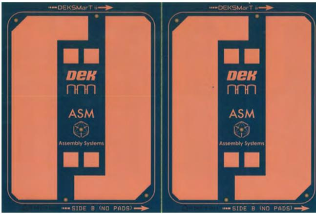
Figure 8: Test PCB, blank bottom side (side B).
