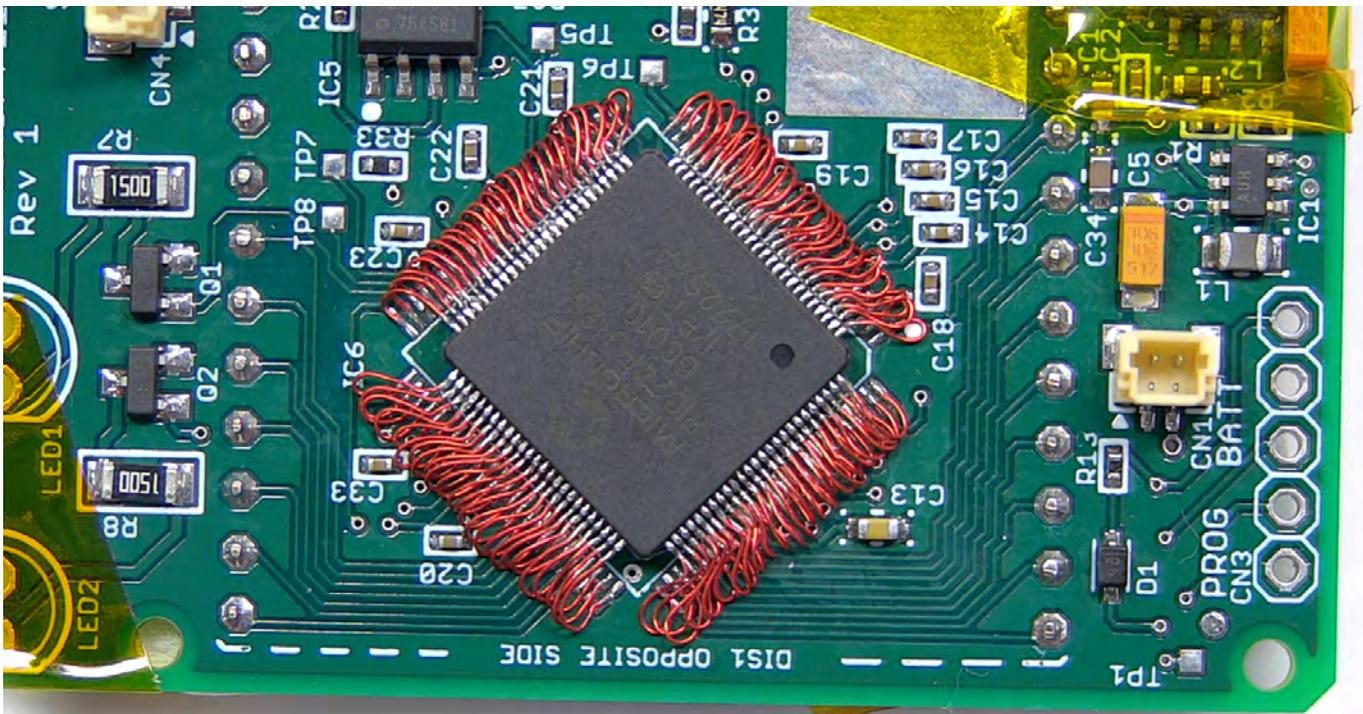
Figure 1: Dead bug attachment of QFP to different pads on a PCB due to a layout problem.
