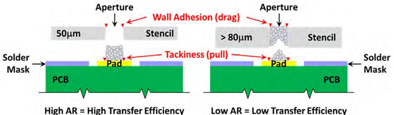
Figure 5: Stencil aperture size influence on paste transfer.
