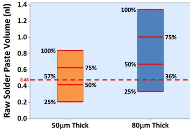
Figure 6: Solder volume transfer efficiency comparison.
