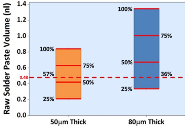
Figure 6: Solder volume transfer efficiency comparison.
