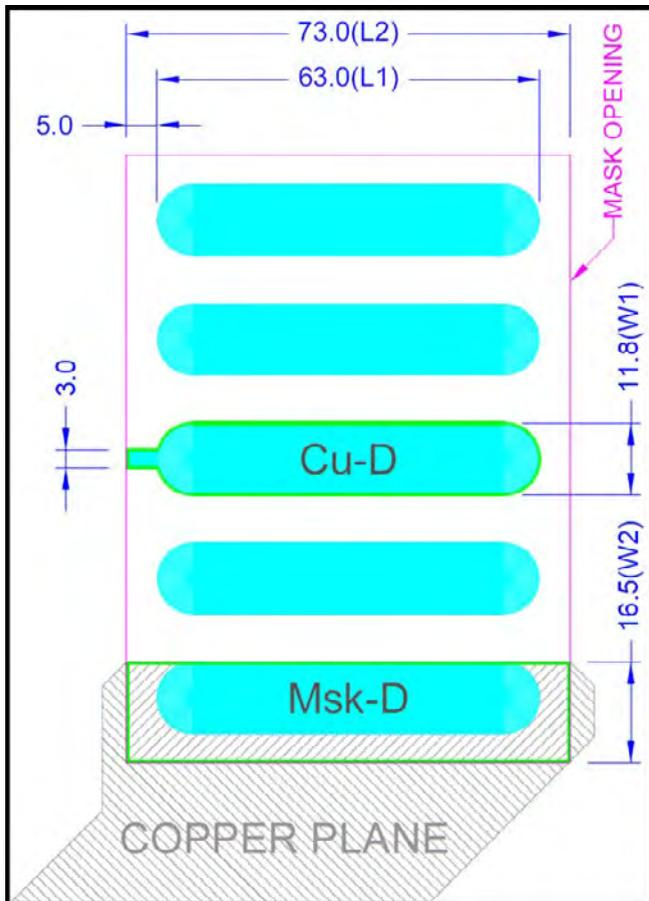
Figure 1: Graphical representation of the pad definitions with example dimensions.
