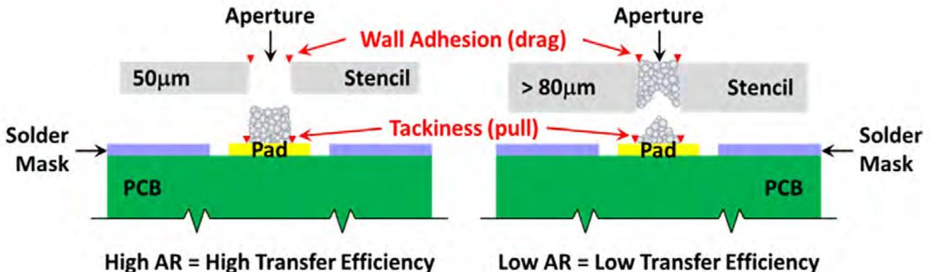
Figure 5: Stencil aperture size influence on paste transfer.
