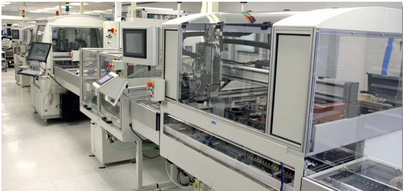
Figure 2: Fully automated test line for implantable electronic modules. Picture courtesy Micro Systems Technologies GmbH.
