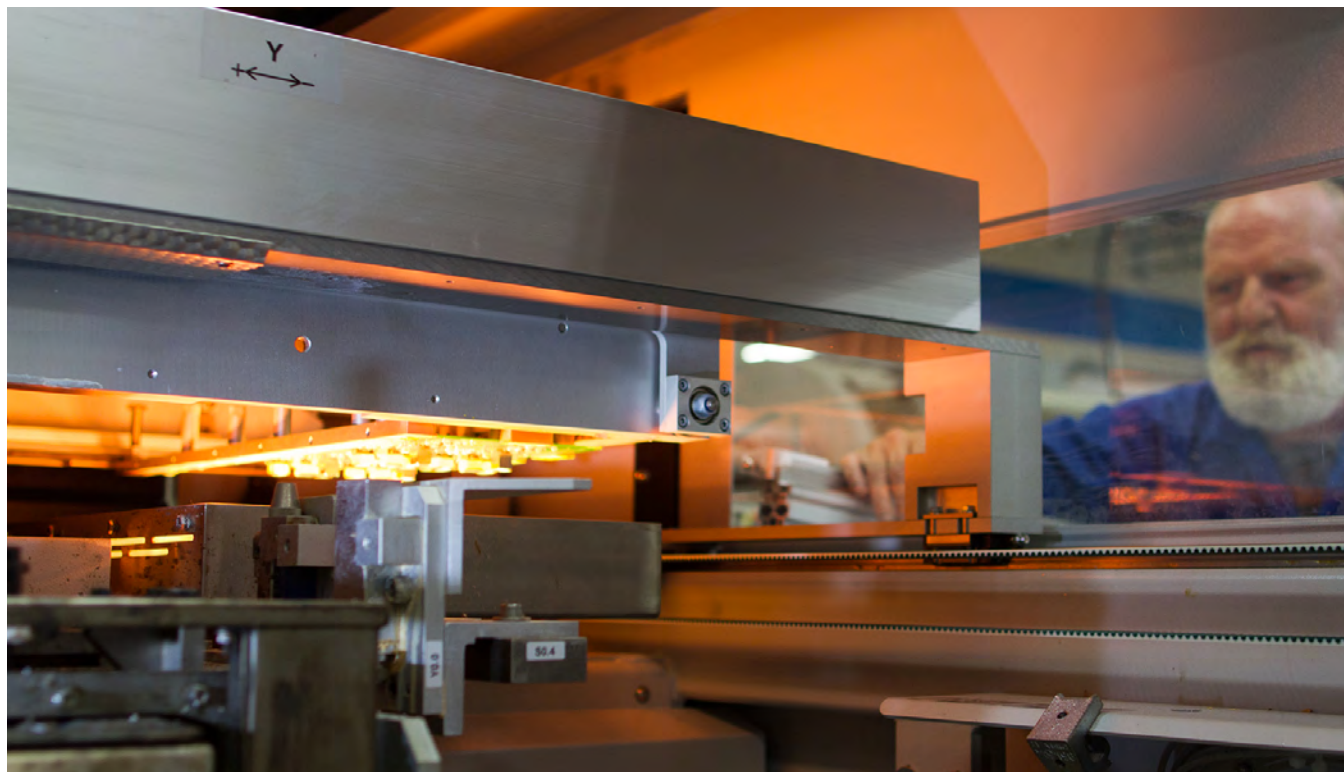
Figure 2: Patrick Reardon, selective solder production specialist, oversees a panel of printed circuit board assemblies during the selective soldering process.
