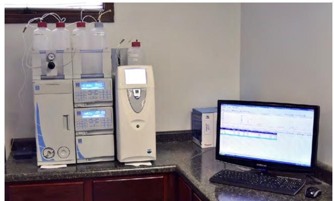
Figure 2: Ion chromatography apparatus.
