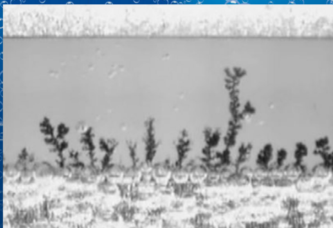
Figure 1: Time-elased footage of dendrite growth on PCB surface.
