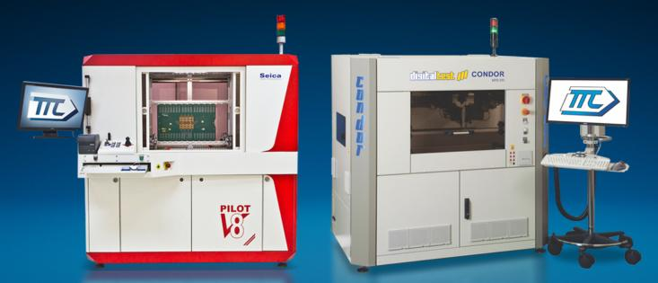
Featuring flying probe test development and board testing by Seica and Digitaltest
