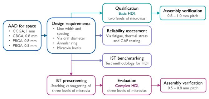
Figure 1: Overall concept for the HDIPCB project.
