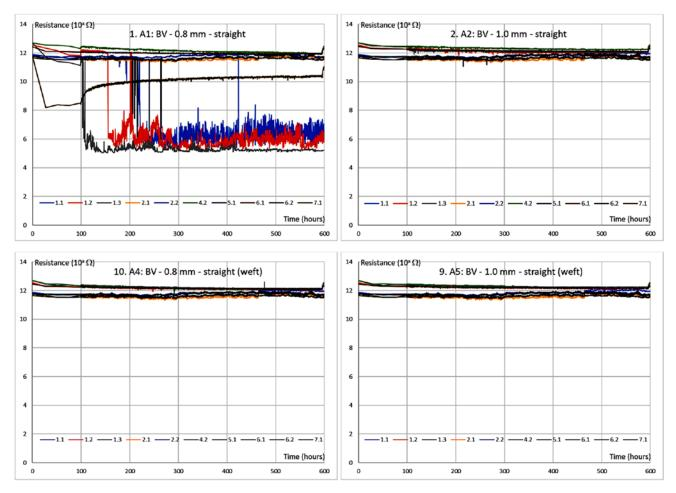
Figure 5: CAF test results for buried vias in a straight configuration with a pitch of 0.8 mm (left) and 1.0 mm (right) for both the warp (upper row) and weft direction (bottom row) of the glass fibers.
