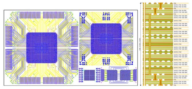
Figure 2: BGA coupon with real and daisy-chain component fanout for 1.0-mm and 0.8-mm pitch component (left) and build-up of the qualification test vehicle (right).
