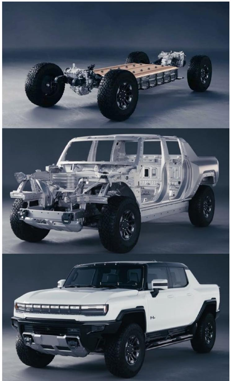
Figure 3: The 2022 GM Hummer EV showing its Ultium EV all-wheel-drive power train and skeleton.
