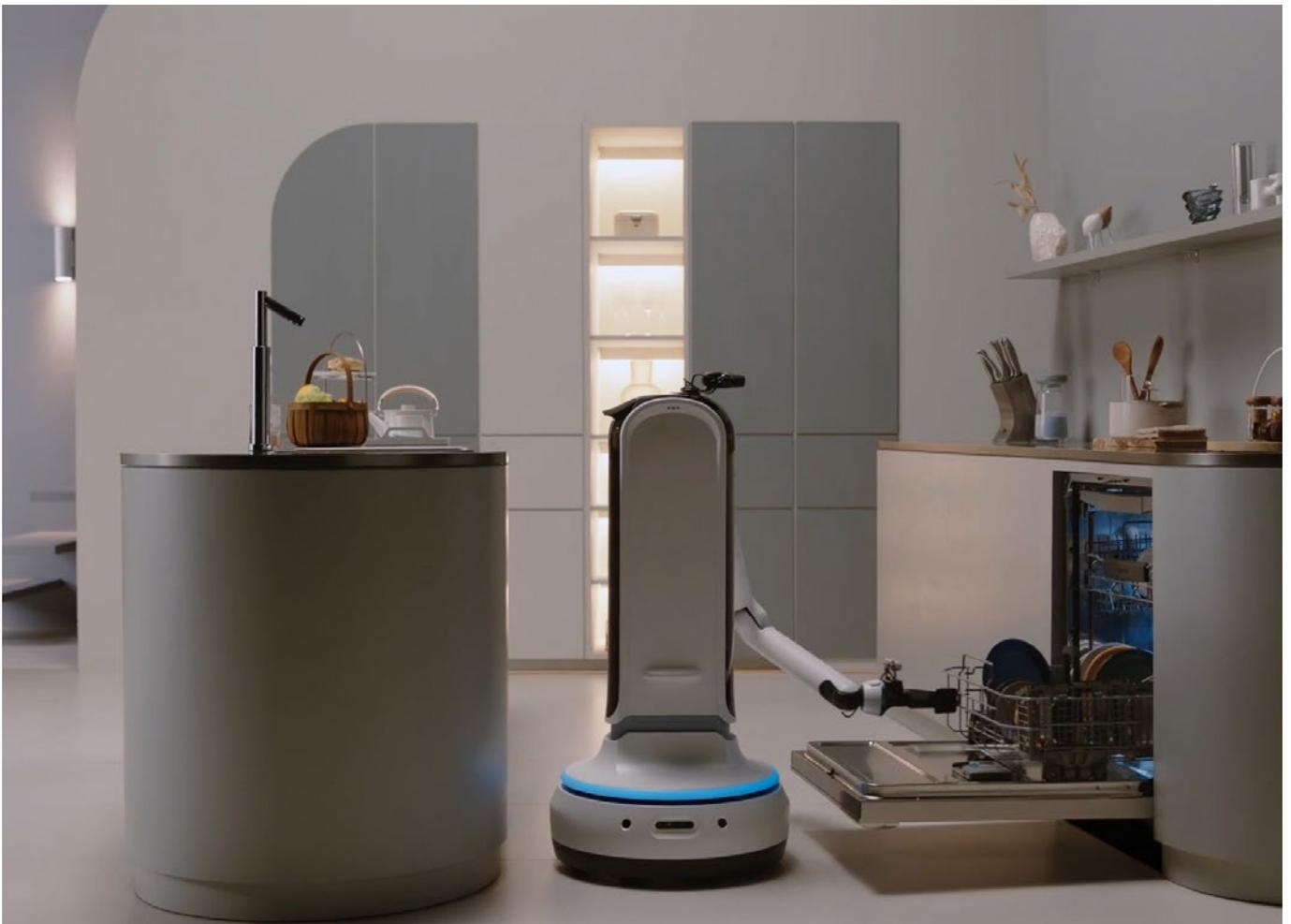
Figure 15: Samsung BOT Handy™ home robot loading the dishwasher using its AI and camera.
