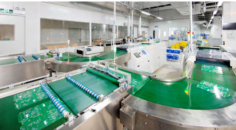
Automated warpage measurement and hole check line.
