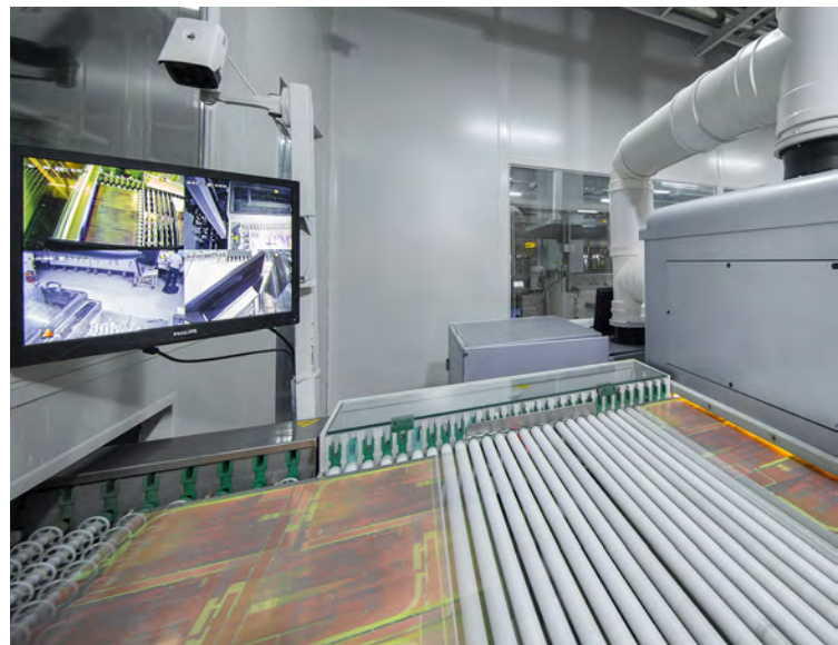
Inline AOI with DES line monitoring.
