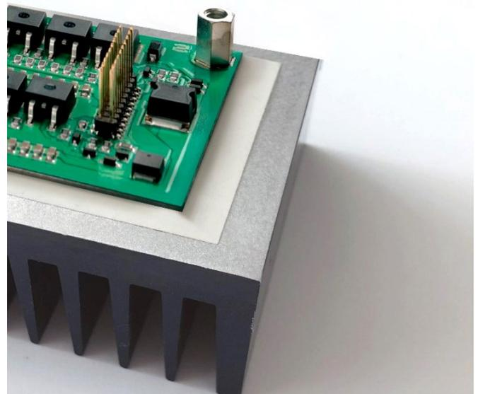
Figure 1: Thermal coupling of a heat source (power module using banks of power components) through a TIM to an external heat sink is an important element in the entire cooling chain that needs to be considered in power electronics.
