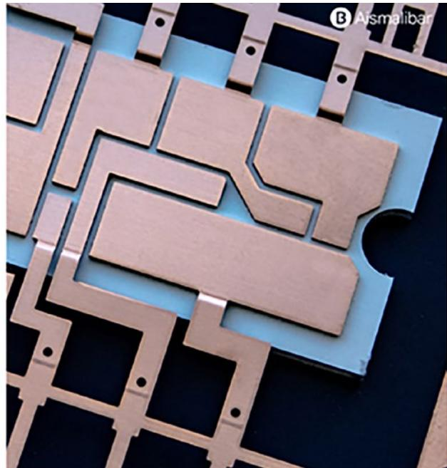
Figure 6: Copper substrate coated with two thermally conductive polymer resins, supplied as a B-stage over a polymerized C-stage layer. (Source: Aismalibar)
