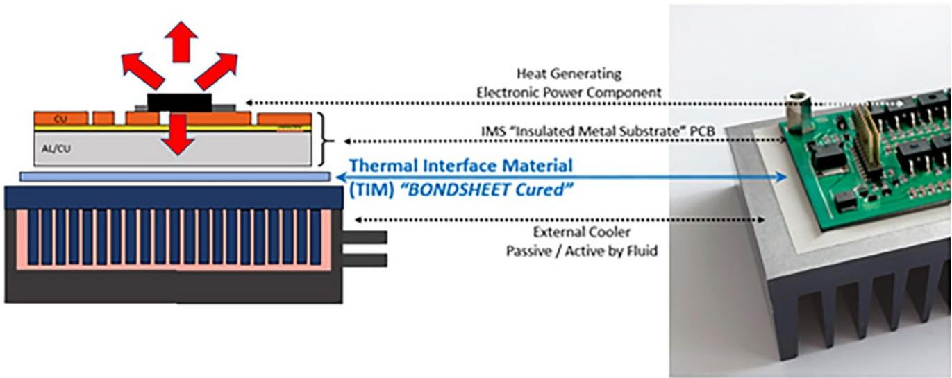
Figure 2: Schematic of a cooling system in power electronics, using the example of an IMS power board, coupled to an aluminum heat sink via TIM. (Source: Aismalibar)
