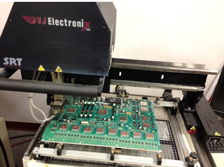
Figure 2: A programmable solder excavation tool.
