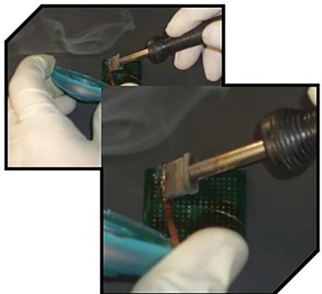
Figure 1: Solder wick being used to remove remnant solder prior to reballing BGA.
