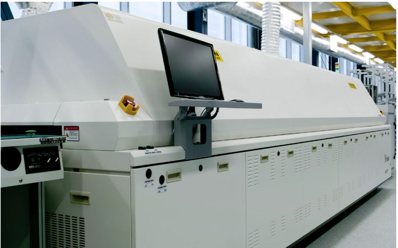
Figure 1: Sue March works on a reflow oven like this one.
