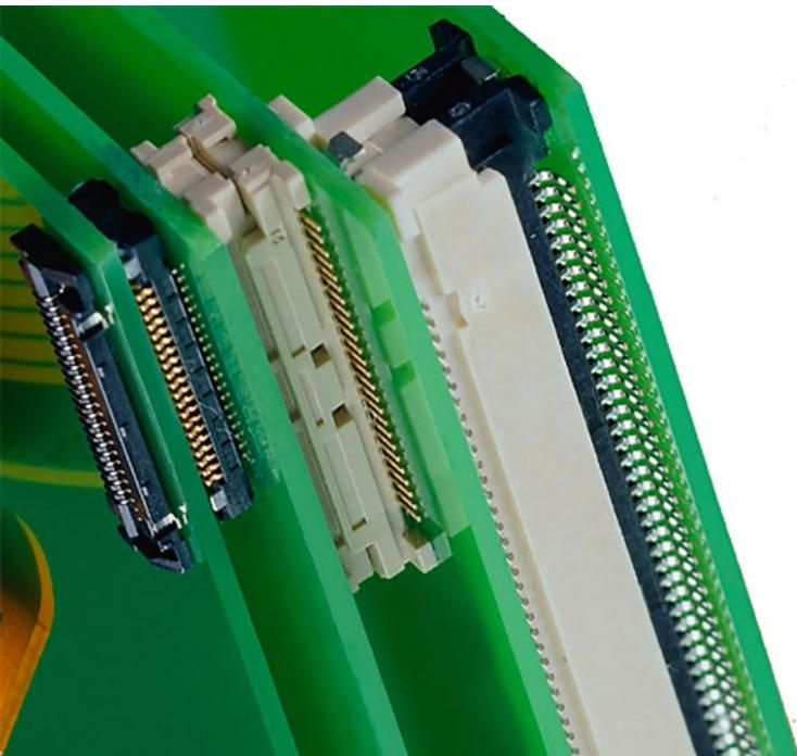
Figure 1: Board-to-board connector.
