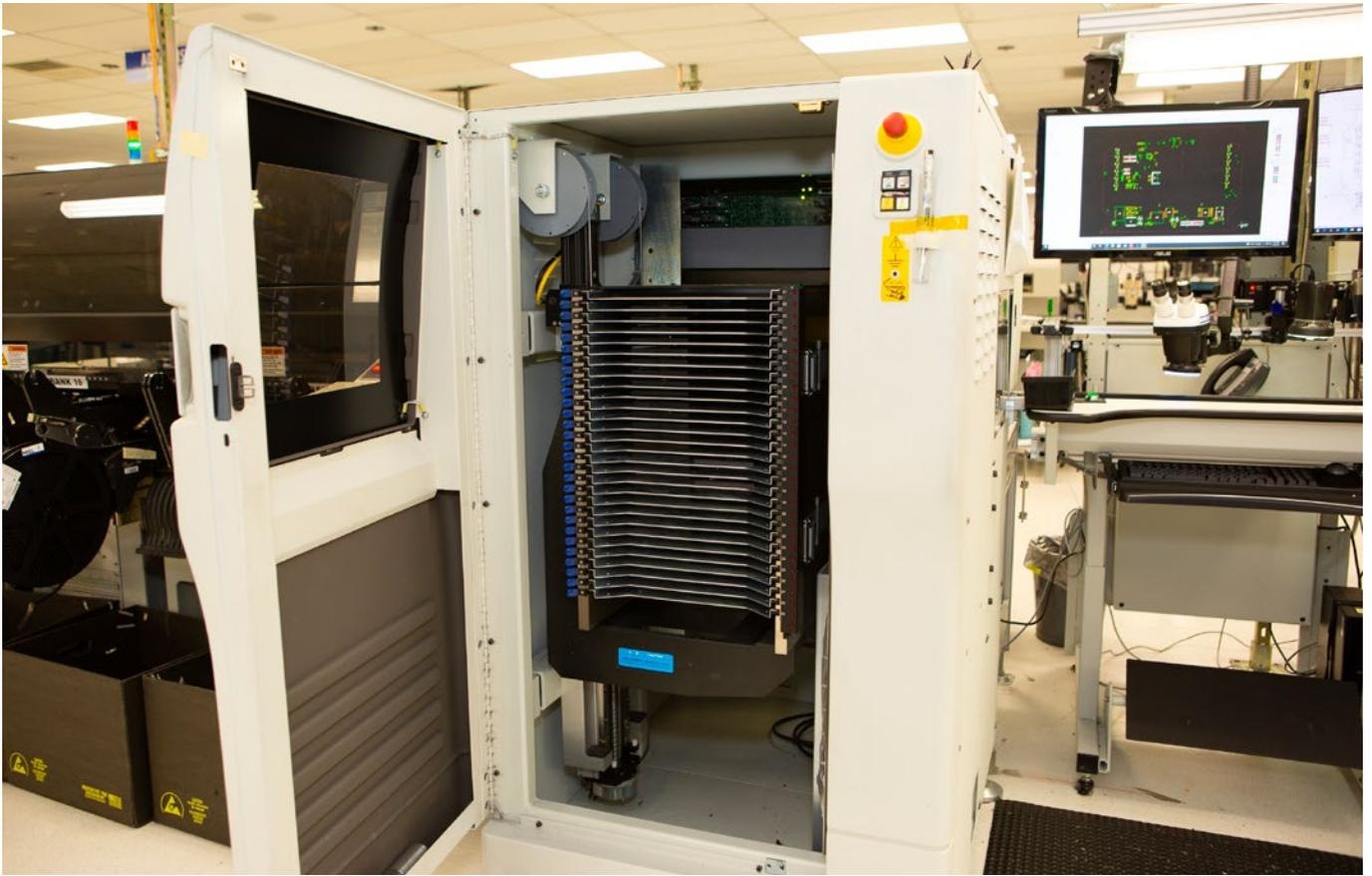
The inside of a random access matrix tray handler showing the elevator and tray handling unit.
