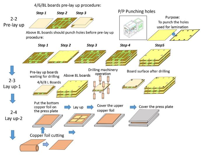
Figure 2: Benchmark detail of the manufacturing process. This example is the multilayer lay-up process.
