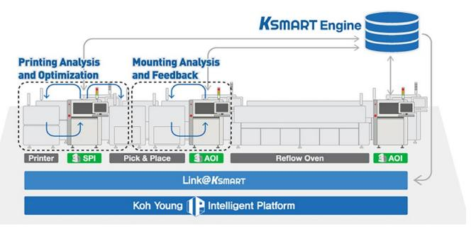
Figure 4: Achieving a smart factory by using 3D inspection process information.
