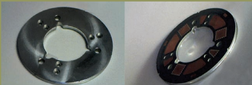
Figure 2. Metalcore PCB with an aluminum base.
