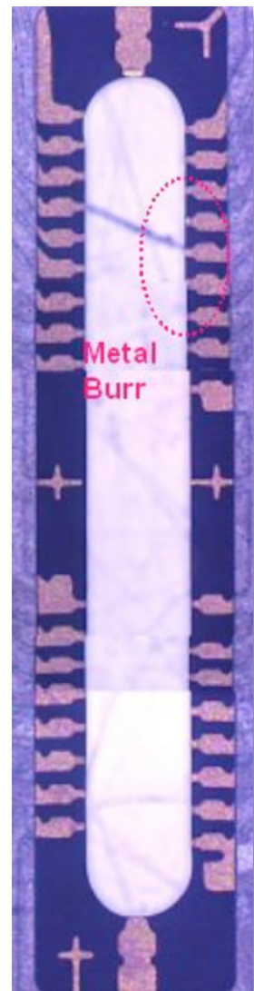
Figure 16: Burr B (electrical short problem).
