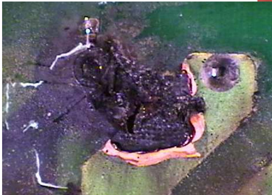
Figure 3: Burnt PCB resulting from arcing, initially caused by dendrites.
