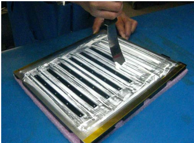
Figure 4: Thermal grease is used to dissipate heat.
