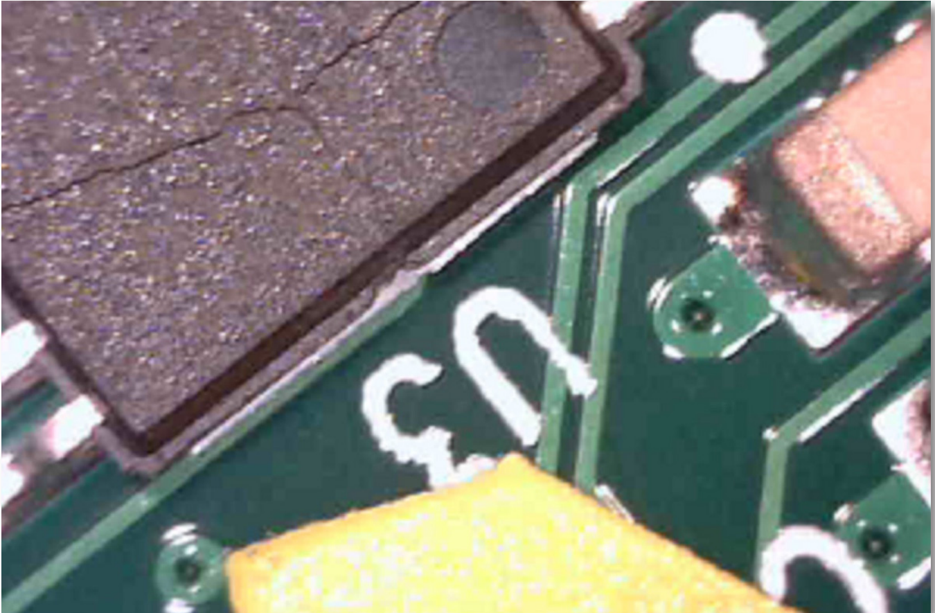
Figure 2: Fractured component due to overheating.
