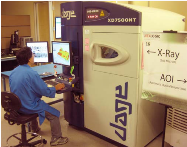
Figure 5: Inspection of complex BGA, QFN, and flip chip packaging demands the use of sophisticated X-ray machines.
