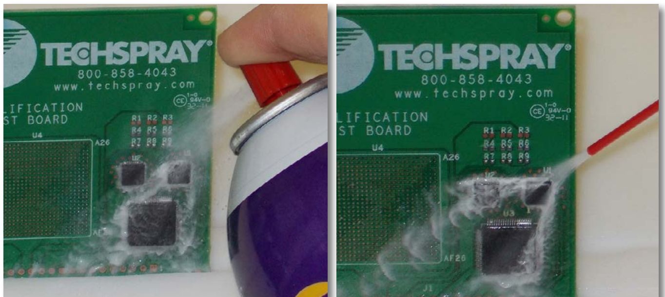
Figure 1: Visual comparison of an aerosol spray without (left) and with a straw attachment.
