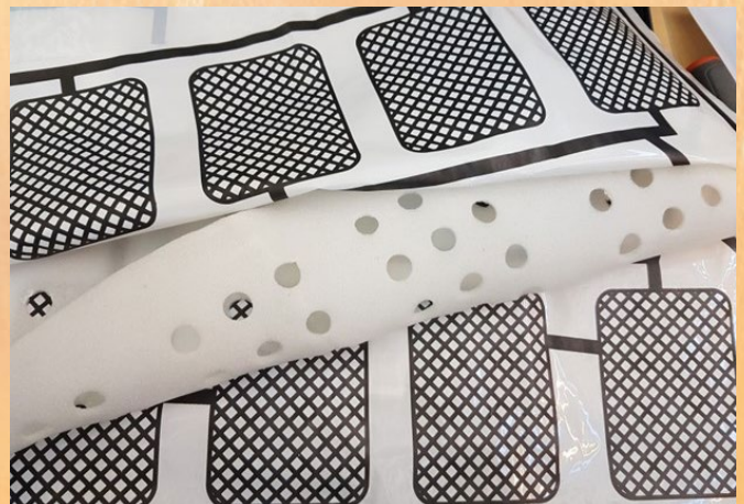
Printed electronics e-textile. (Source: IPC-WP-025, courtesy of Loomia)
