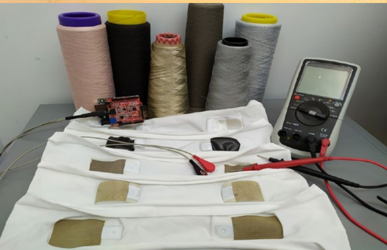
Electrodes for wearables systems. (Source: ENSAIT)
