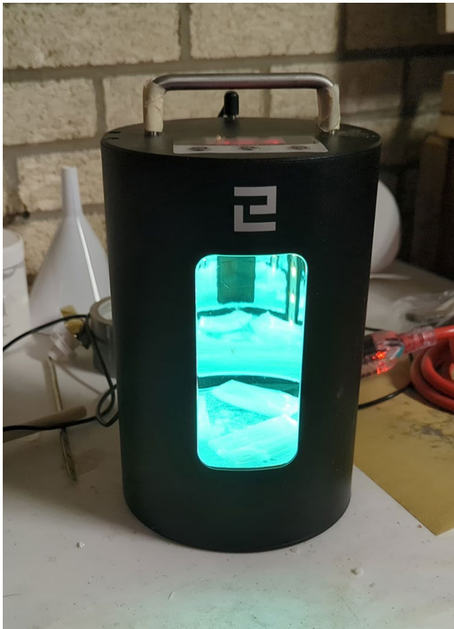
The UV chamber allows for fast curing of prints.
